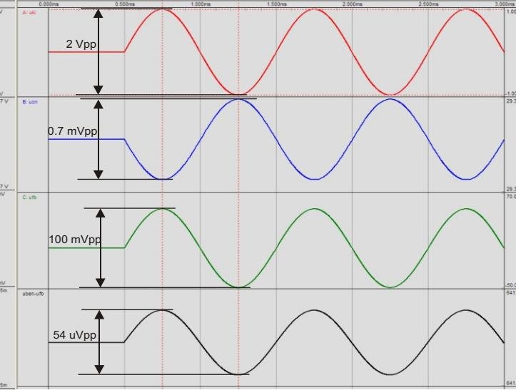
$$1/A_V = 1/A_U + \frac{R_1}{R_1+R_2}$$
