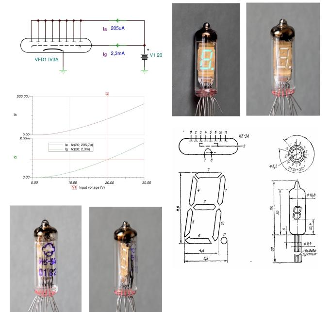
A VFD operates on the principle of <u>cathodoluminescence</u>, roughly similar to a <u>cathode ray</u> <u>tube</u>, but operating at much lower voltages. For more info see:<u>IV-3A DataSheet</u>.
