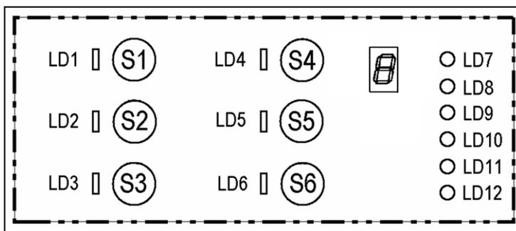
Control panel with the maximum configuration with display: - HORIZONTAL Version
