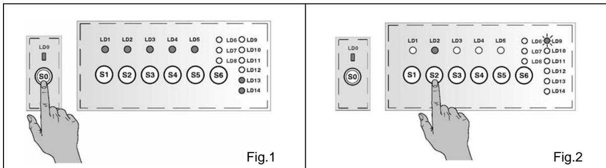
1. When the appliance is switched on with S0 button (fig.1) the pre-selection phase is indicated
