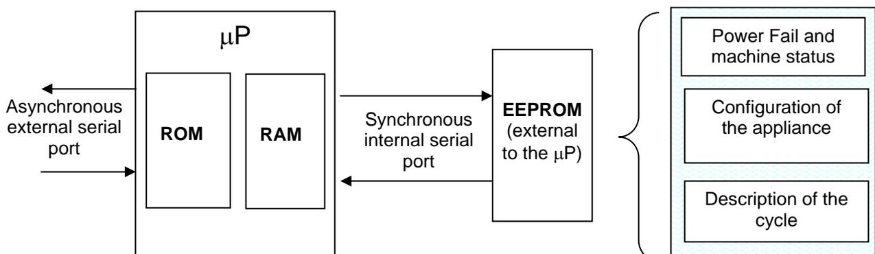
The main circuit board features an EEPROM memory (external to the microprocessor) which stores in memory data relative to the configuration, description of the cycle, cycle status in case of a power failure, and any alarm conditions.
