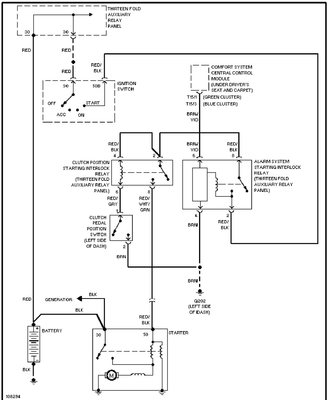
1.9L Turbo Diesel, Starting Circuit, M/T
