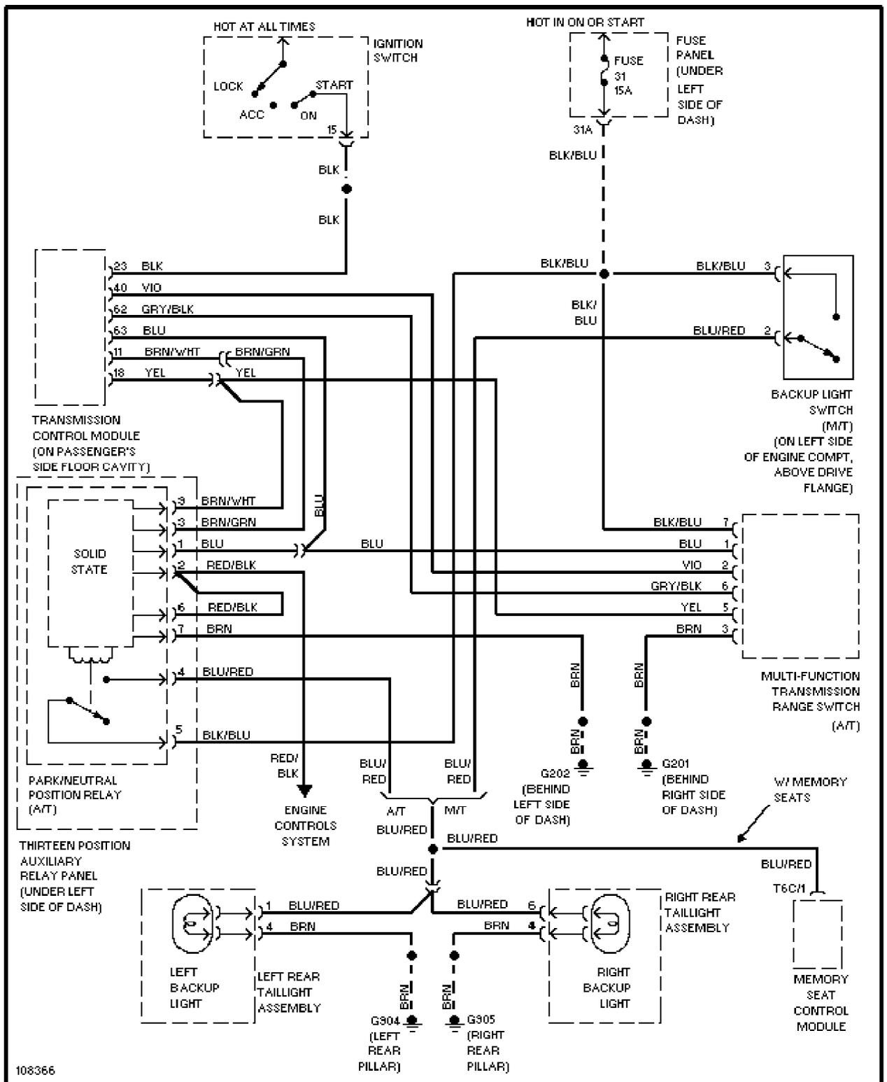
1.9L Turbo Diesel, Back-up Lamps Circuit
