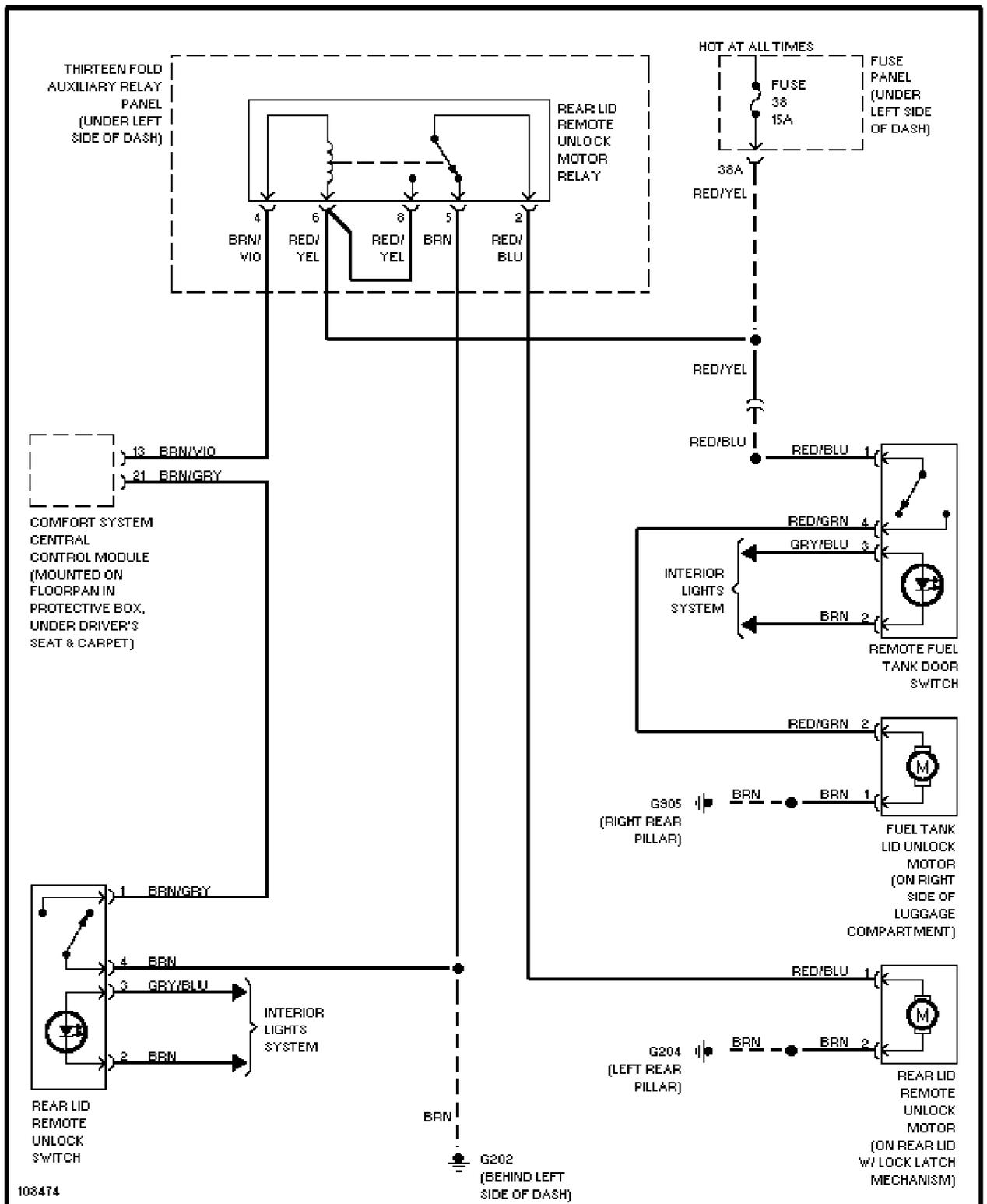
Trunk & Fuel Door Release Circuit
