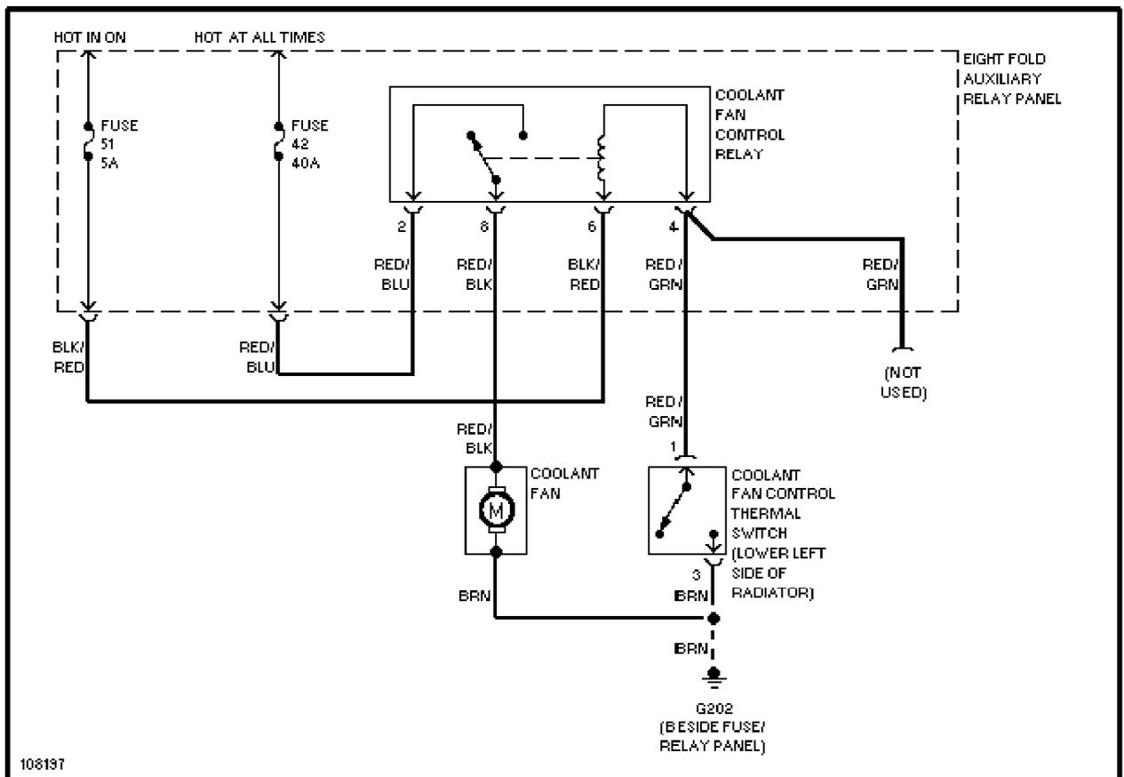
Single Speed Cooling Fan Circuit
