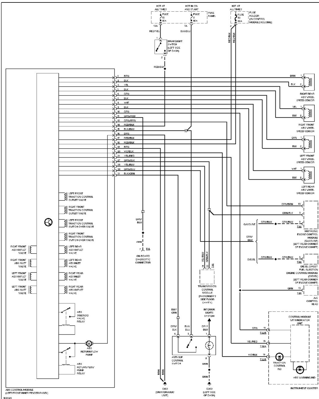
Anti-lock Brake Circuits, W/ Traction Control
