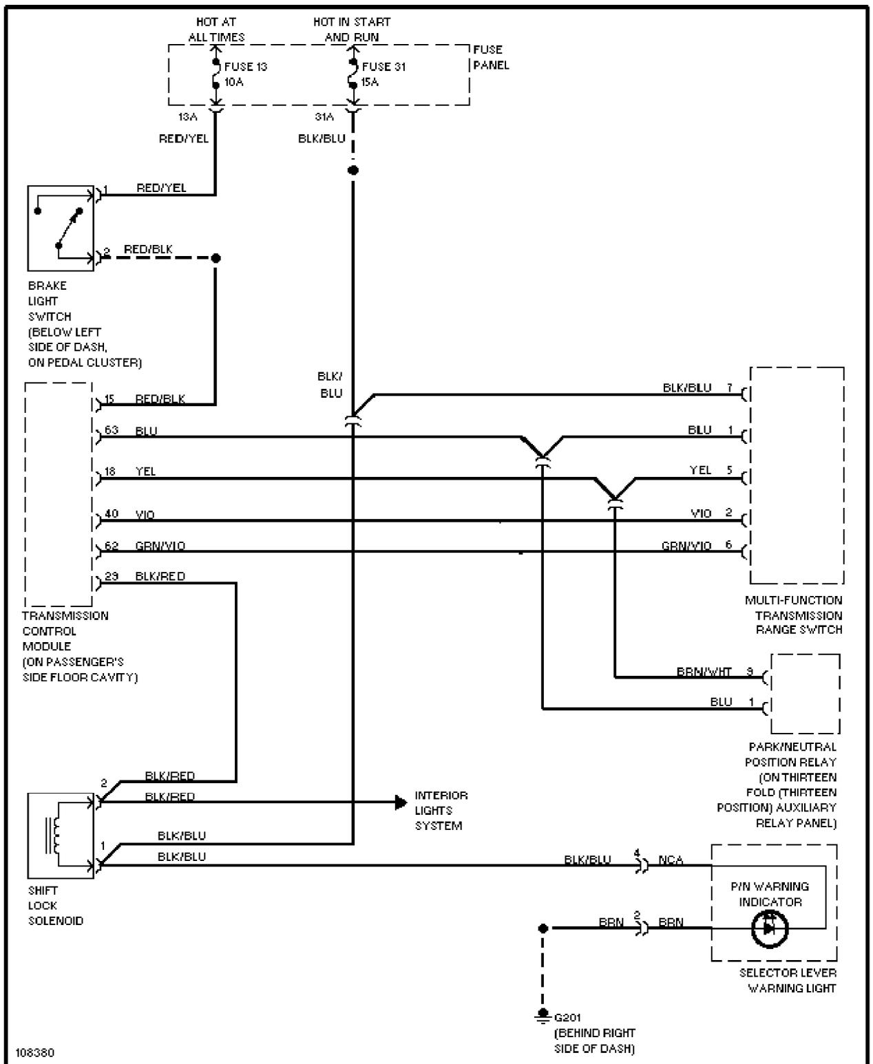
1.9L Turbo Diesel, Shift Interlock Circuit
