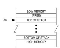
To implement stack growth from low memory to high memory, use (An) + to push data on the stack and -(An) to pull data from the stack. After either a push or pull operation, the address register points to the next available space on the stack.
