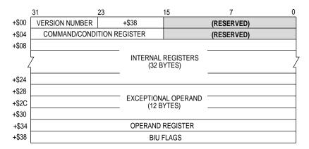
Figure B-19. MC68882 Idle Stack Frame
