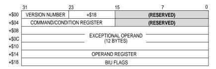
Figure B-17. MC68881 Idle Stack Frame
