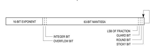
Figure 3-1. Intermediate Result Format
