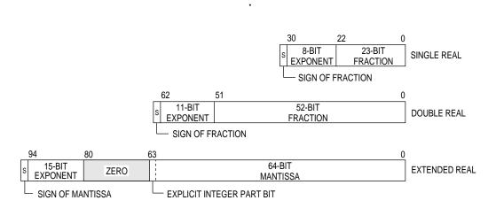
Figure 1-12. Binary Floating-Point Data Formats
