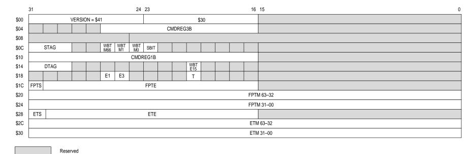
Figure B-22. MC68040 Unimplimented Instruction Stack Frame
