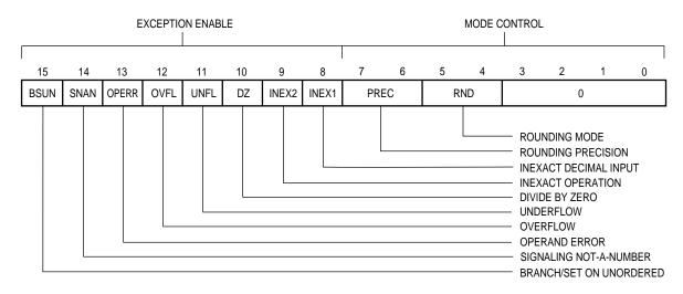
Figure 1-3. Floating-Point Control Register
