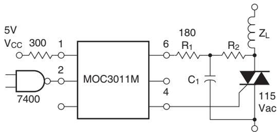
NOTE: Circuit supplies 25mA drive to gate of triac at  $V_{in} = 25V$  and  $T_A < 70^\circ C$
