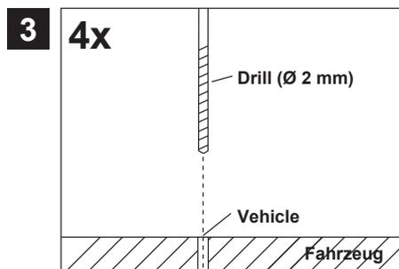
Put the GP800 aside and then drill the holes for the mounting screws at the before marked locations.
