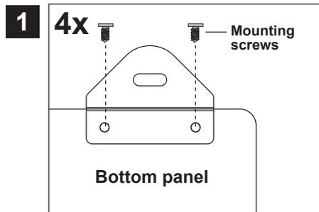
There are at each corner two predrilled screw holes on the GP800's bottom panel. Please attach there the four supplied mounting brackets with the eight mounting screws.
