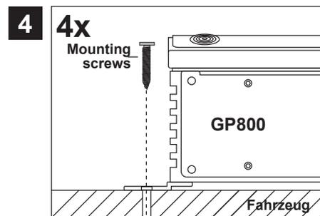
Then uphold the GP800 to the chosen position and fix the screws through the holes of the mounting brackets into the drilled screwholes.
