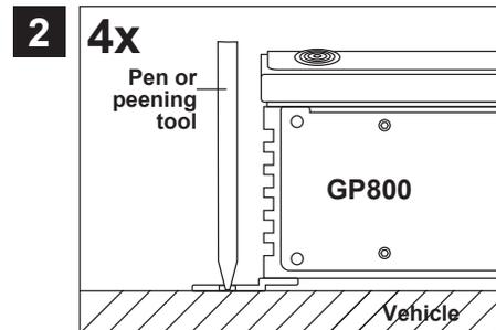
Uphold the GP800 to the chosen mounting location in the vehicle, after you have attached the mounting brackets. Then mark the four drill holes with a appropriate pen or peening tool and lead through the mounting openings.
