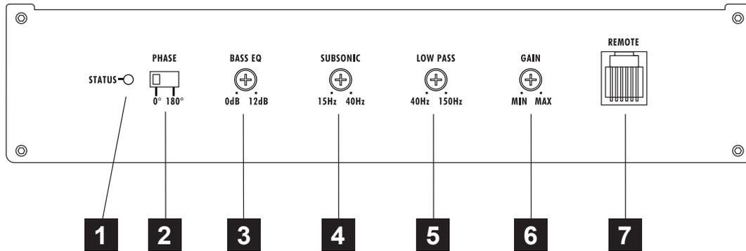
**1** **STATUS LED.** If the LED lights up green, the amplifier is ready for operation. If the LED lights up red, a malfunction is indicated. Check in this case the chapter **TROUBLE SHOOTING**.
