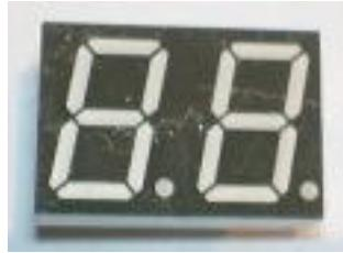
The digits are common anode (+). The pinout is shown below (top view!).
