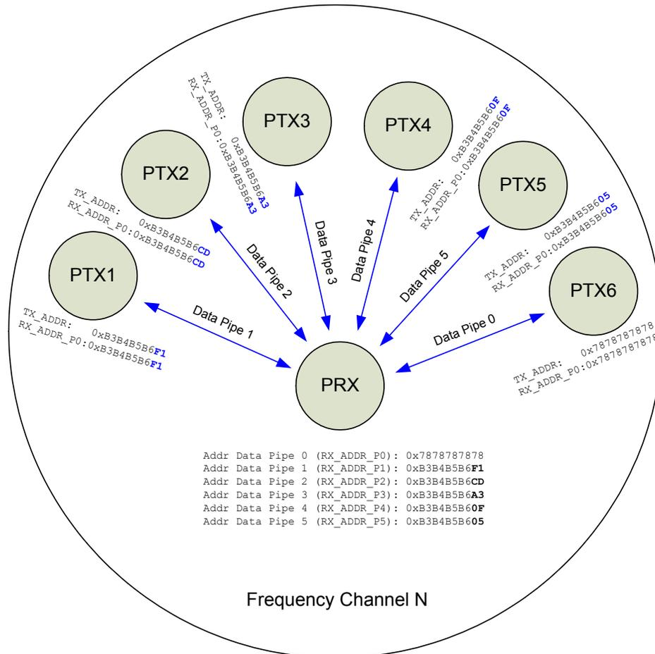
Figure 12. Example of data pipe addressing in MultiCeiver™
