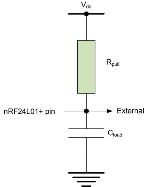
Figure 26.  $R_{pull}$  and  $C_{load}$
