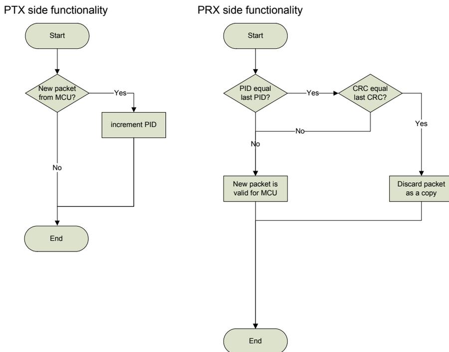
Figure 6. PID generation/detection
