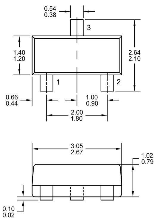
1. All linear dimensions are in millimeters.
