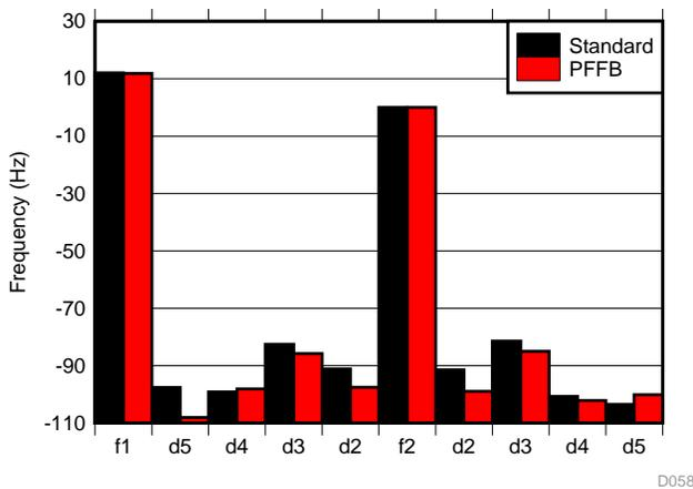
Figure 91. SMPTE IMD Distortion Product Ratio at 1 W
