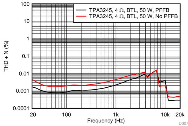
**Figure 9. THD+N vs Frequency at 50 W**
