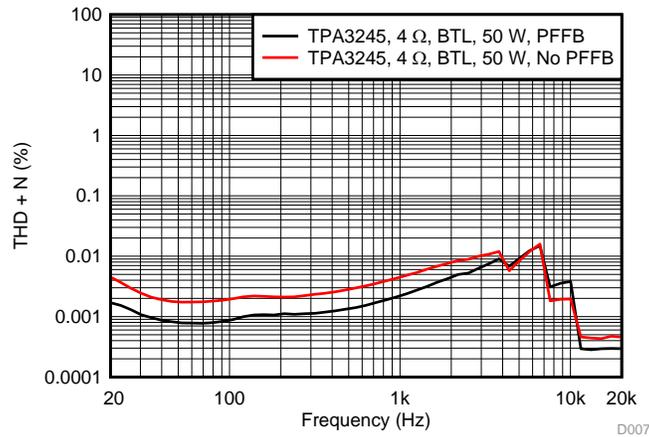
Figure 45. THD+N vs Frequency at 50 W
