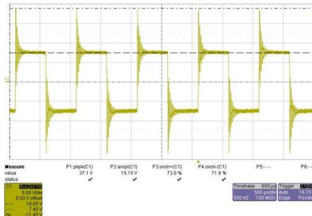
**Figure 19. TPA3245 PFFB 1-kHz Square Wave Open Response**
