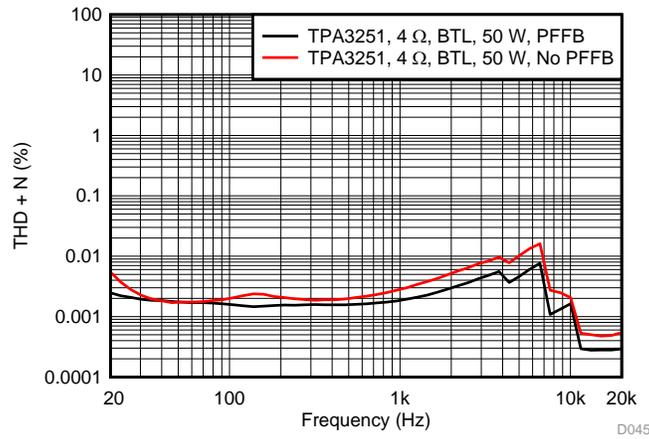
Figure 75. THD+N vs Frequency at 50 W
