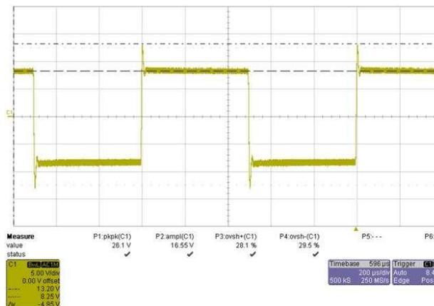
Figure 22. TPA3245 PFFB 1-kHz Square Wave 8-Ω Response
