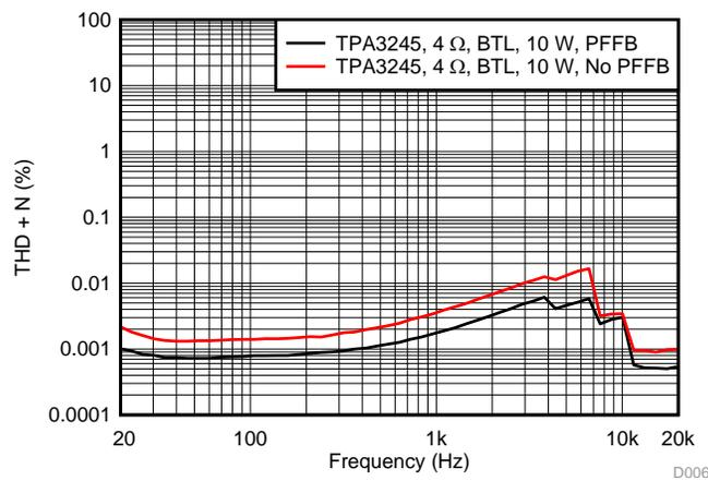
**Figure 44. THD+N vs Frequency at 10 W**
