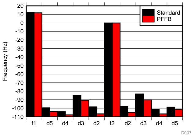
Figure 46. SMPTE IMD Distortion Product Ratio at 1 W
