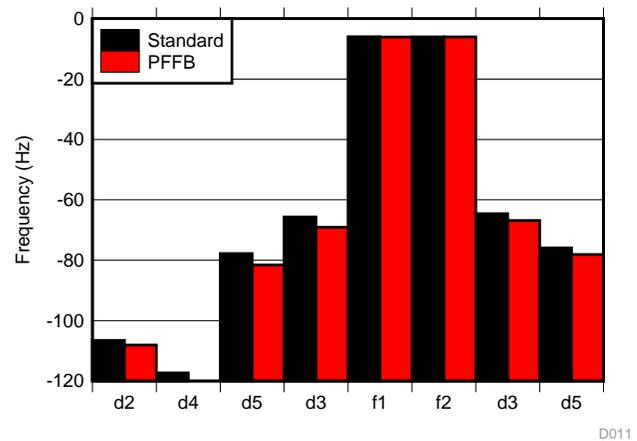
Figure 50. CCIF IMD Distortion Product Ratio at 10 W
