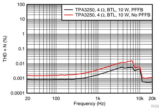
Figure 59. THD+N vs Frequency at 10 W
