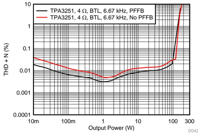
Figure 72. THD+N vs Power at 6.67 kHz
