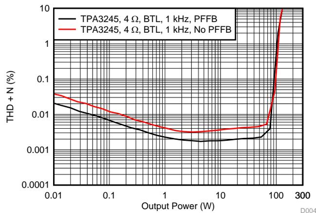
**Figure 40. THD+N vs Power at 1 kHz**
