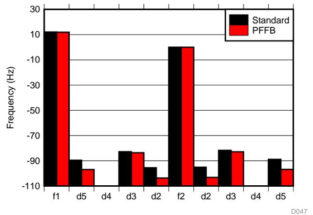
Figure 77. SMPTE IMD Distortion Product Ratio at 10 W
