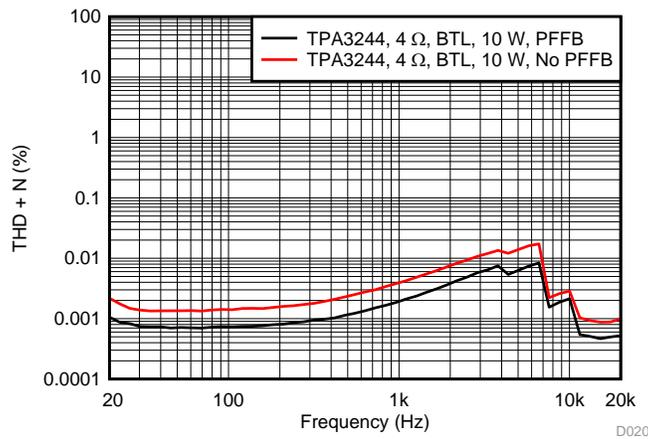
**Figure 29. THD+N vs Frequency at 10 W**
