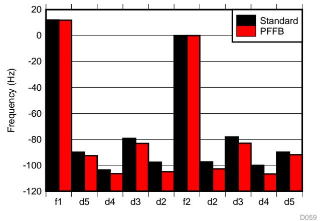
Figure 92. SMPTE IMD Distortion Product Ratio at 10 W
