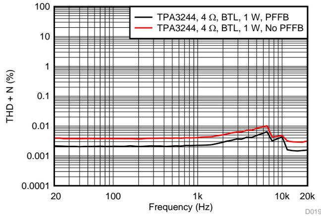
**Figure 28. THD+N vs Frequency at 1 W**
