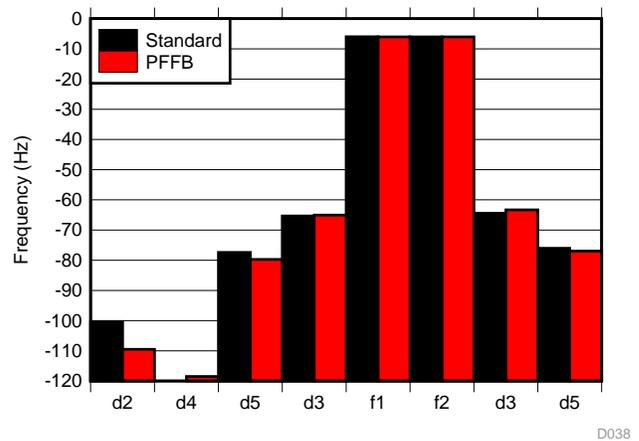
Figure 65. CCIF IMD Distortion Product Ratio at 10 W
