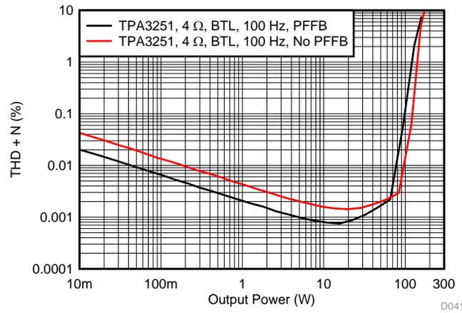
Figure 71. THD+N vs Power at 100 Hz
