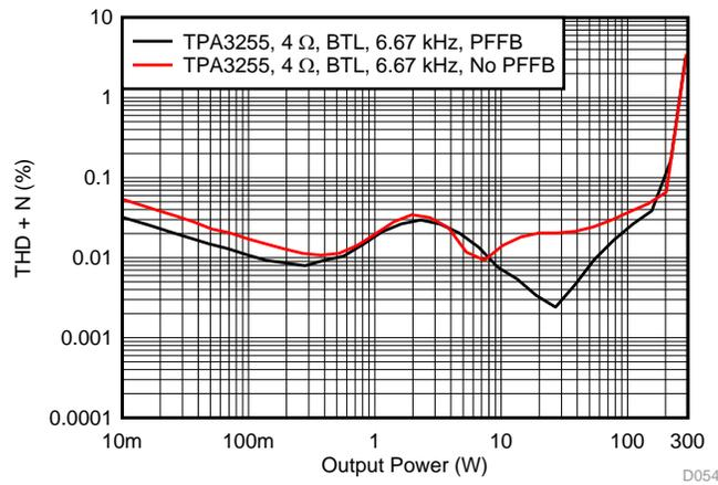
Figure 87. THD+N vs Power at 6.67 kHz
