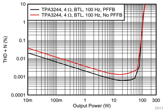
**Figure 26. THD+N vs Power at 100 Hz**
