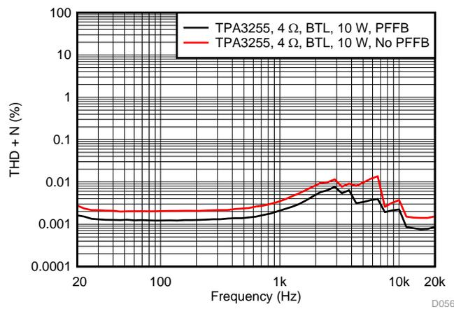
Figure 89. THD+N vs Frequency at 10 W
