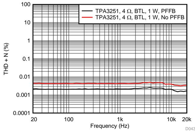
Figure 73. THD+N vs Frequency at 1 W
