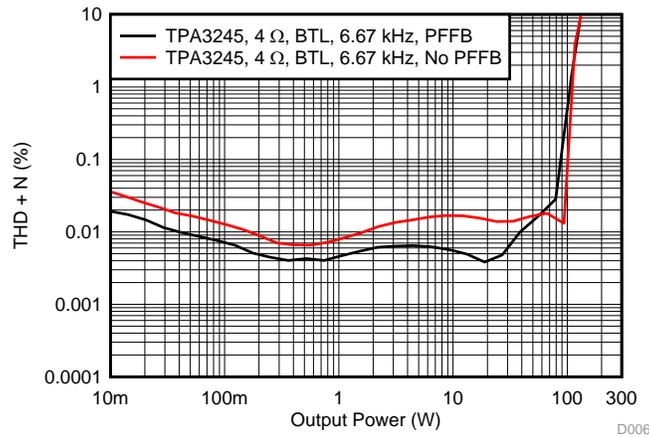
**Figure 6. THD+N vs Power at 6.67 kHz**
