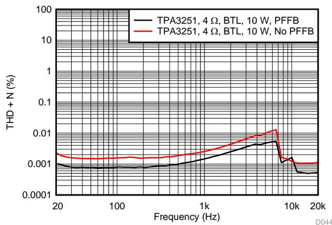
Figure 74. THD+N vs Frequency at 10 W
