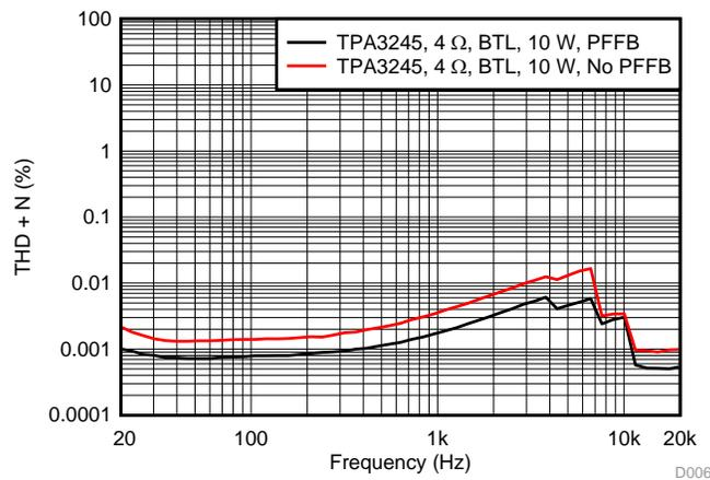
Figure 8. THD+N vs Frequency at 10 W
