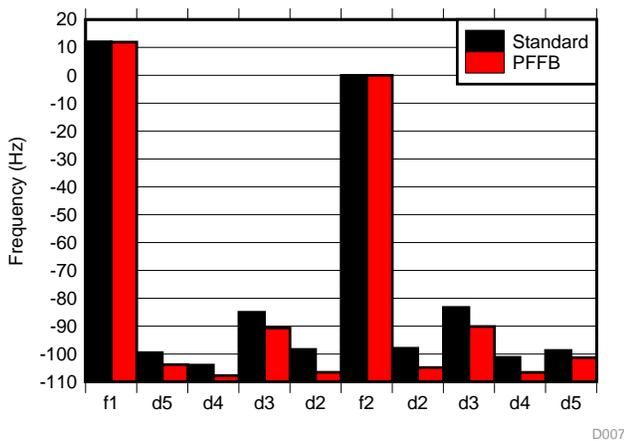
Figure 11. SMPTE IMD Distortion Product Ratio at 1 W
