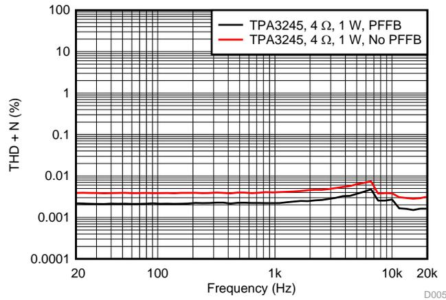
**Figure 43. THD+N vs Frequency at 1 W**
