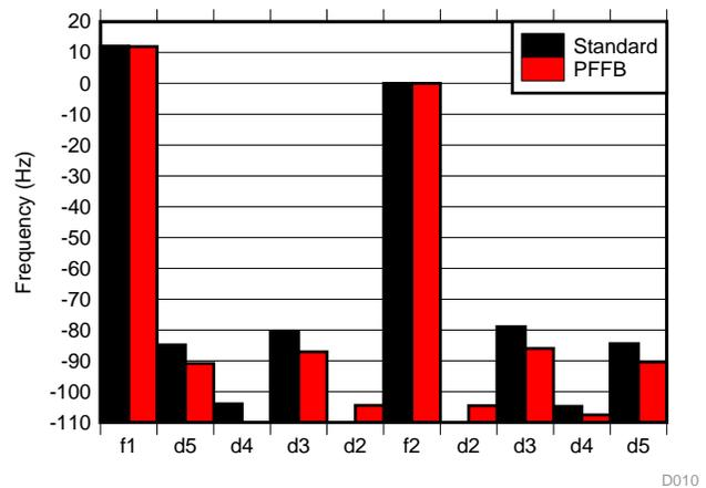
Figure 12. SMPTE IMD Distortion Product Ratio at 10 W
