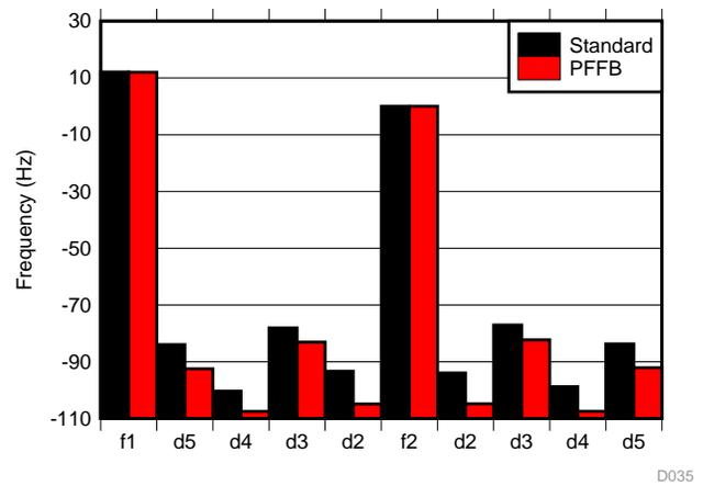
Figure 62. SMPTE IMD Distortion Product Ratio at 10 W
