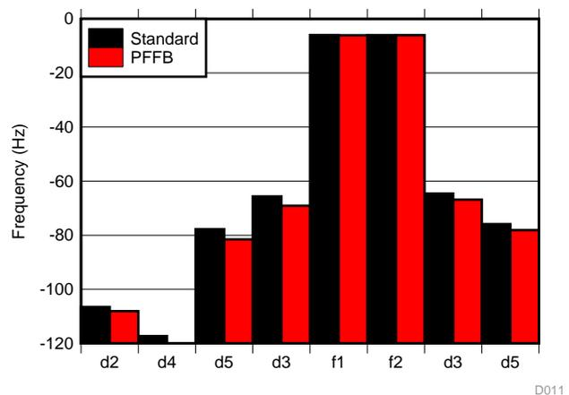
Figure 15. CCIF IMD Distortion Product Ratio at 10 W
