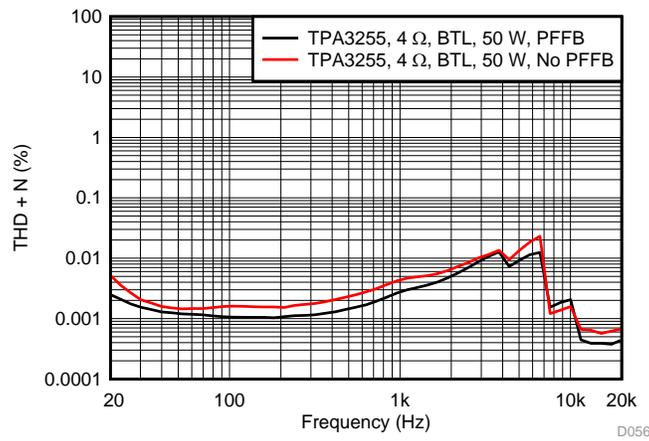
Figure 90. THD+N vs Frequency at 50 W
