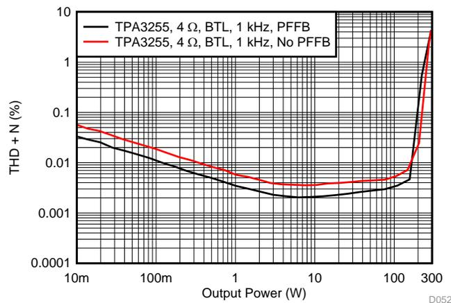
**Figure 85. THD+N vs Power at 1 kHz**
