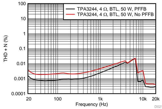
Figure 30. THD+N vs Frequency at 50 W
