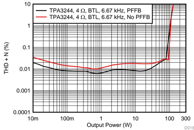
**Figure 27. THD+N vs Power at 6.67 kHz**
