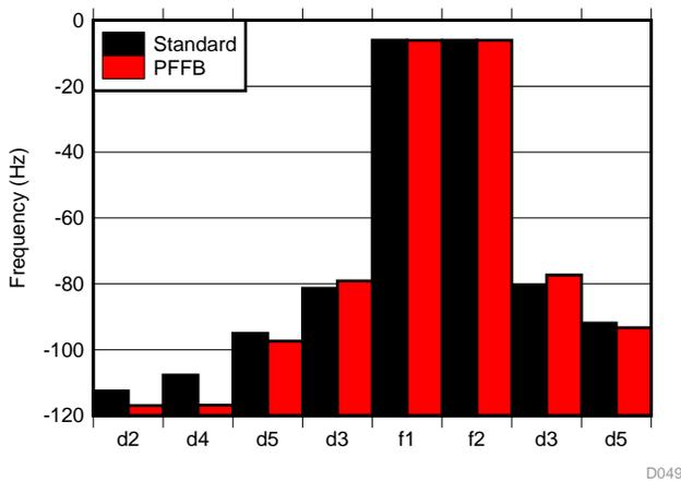
Figure 79. CCIF IMD Distortion Product Ratio at 1 W
