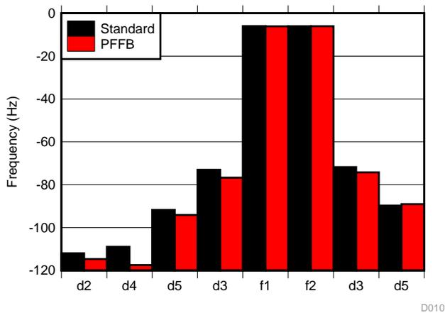
Figure 49. CCIF IMD Distortion Product Ratio at 1 W
