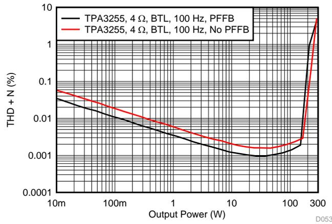
Figure 86. THD+N vs Power at 100 Hz
