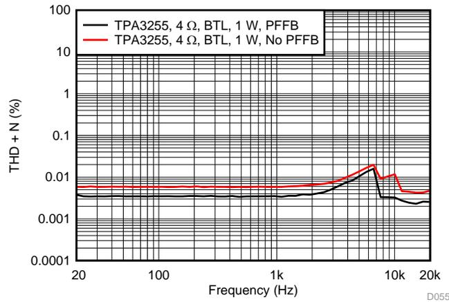
Figure 88. THD+N vs Frequency at 1 W
