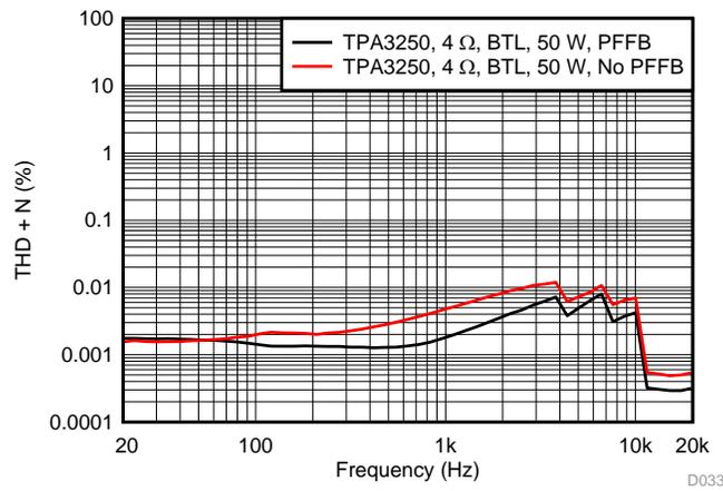
Figure 60. THD+N vs Frequency at 50 W
