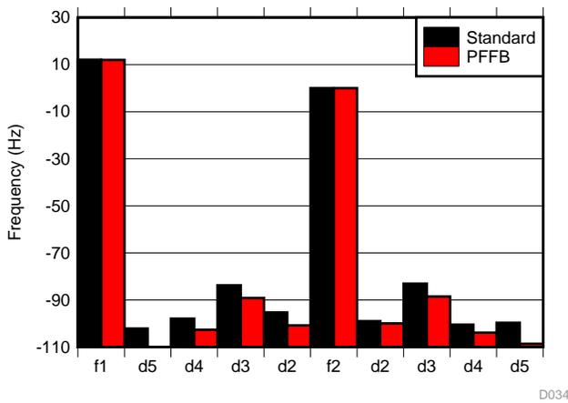
Figure 61. SMPTE IMD Distortion Product Ratio at 1 W
