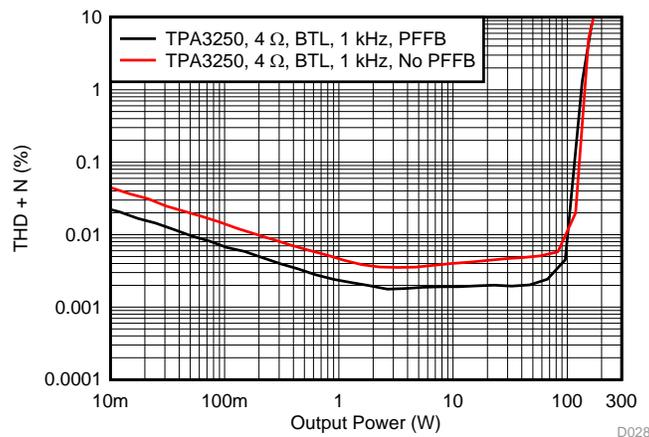
**Figure 55. THD+N vs Power at 1 kHz**
