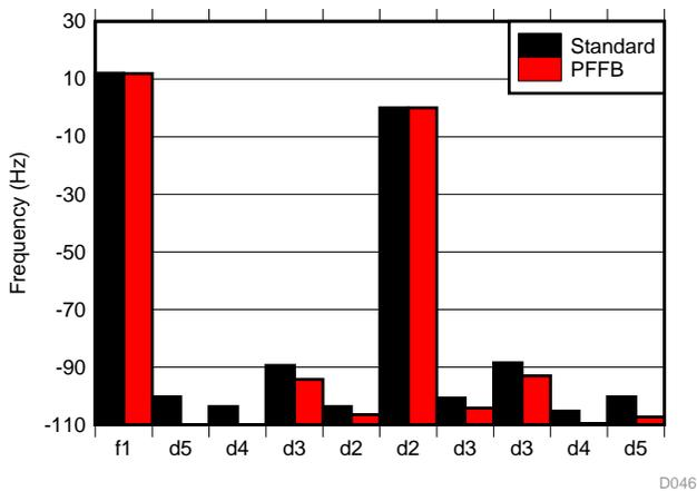
Figure 76. SMPTE IMD Distortion Product Ratio at 1 W
