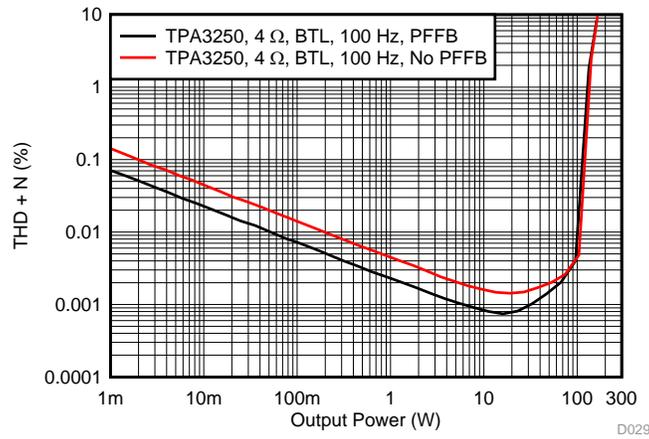
Figure 56. THD+N vs Power at 100 Hz
