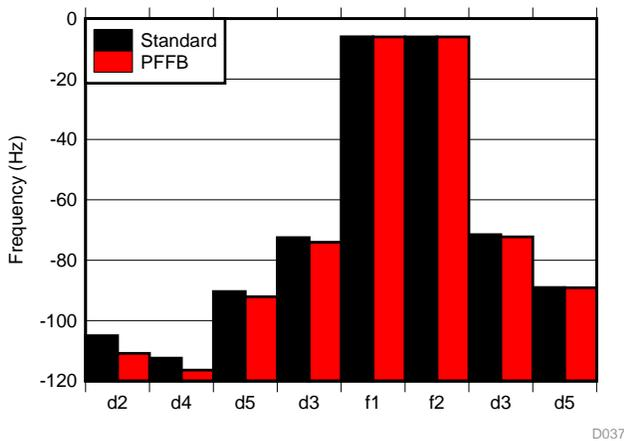
Figure 64. CCIF IMD Distortion Product Ratio at 1 W
