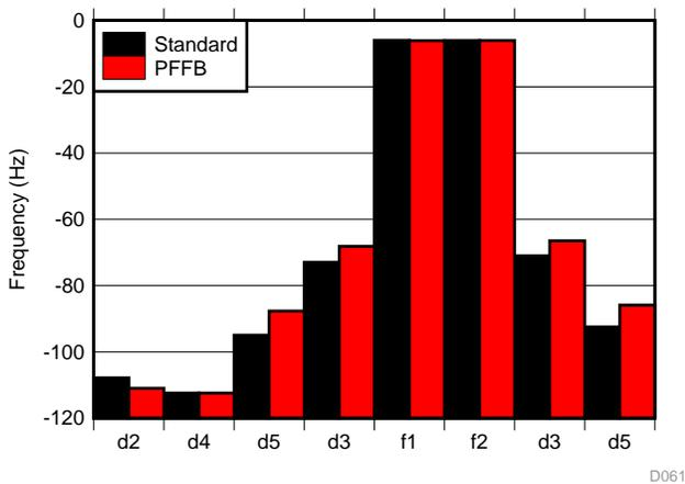
Figure 94. CCIF IMD Distortion Product Ratio at 1 W
