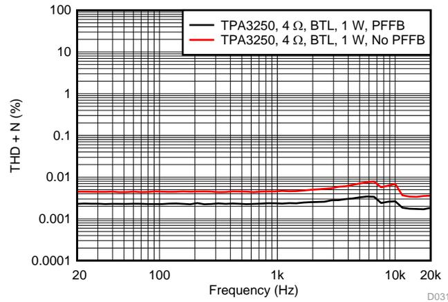
Figure 58. THD+N vs Frequency at 1 W
