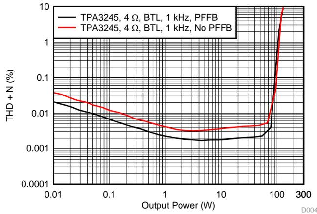
Figure 4. THD+N vs Power at 1 kHz
