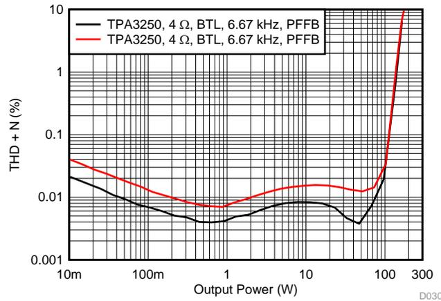
Figure 57. THD+N vs Power at 6.67 kHz
