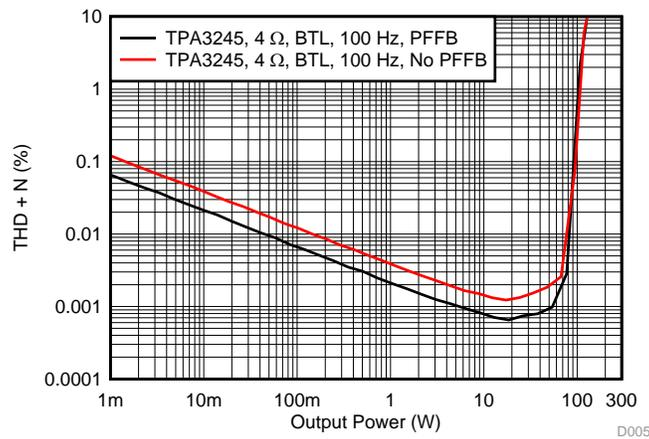
**Figure 41. THD+N vs Power at 100 Hz**
