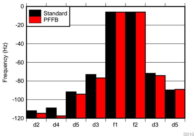
Figure 14. CCIF IMD Distortion Product Ratio at 1 W
