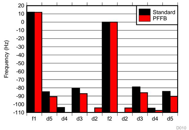
Figure 47. SMPTE IMD Distortion Product Ratio at 10 W
