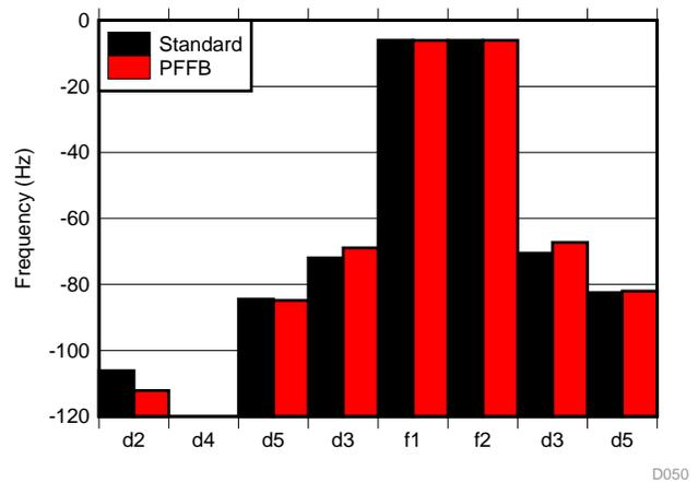
Figure 80. CCIF IMD Distortion Product Ratio at 10 W
