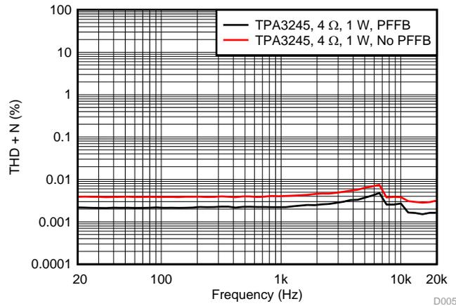
Figure 7. THD+N vs Frequency at 1 W
