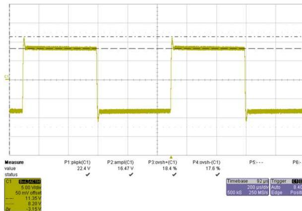
Figure 21. TPA3245 PFFB 1-kHz Square Wave 4-Ω Response
