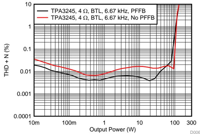
**Figure 42. THD+N vs Power at 6.67 kHz**
