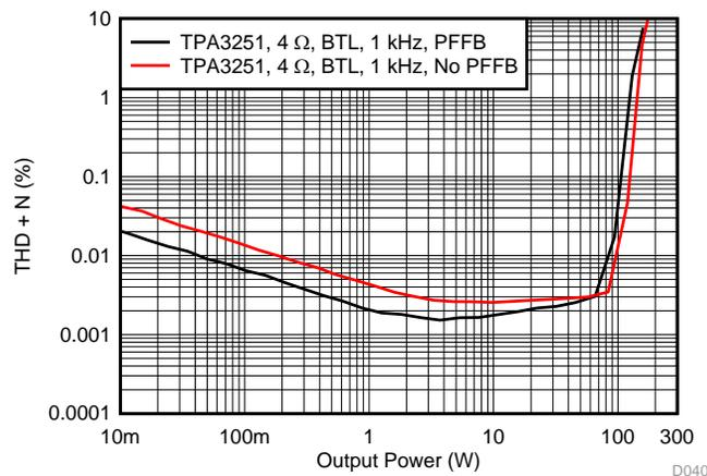
**Figure 70. THD+N vs Power at 1 kHz**
