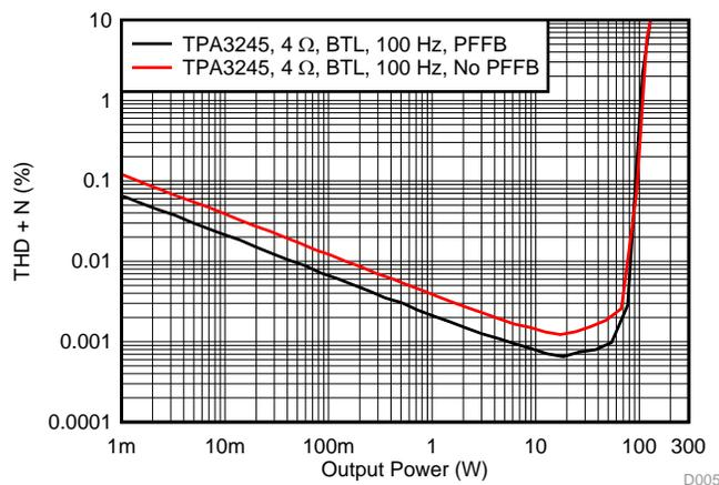
Figure 5. THD+N vs Power at 100 Hz
