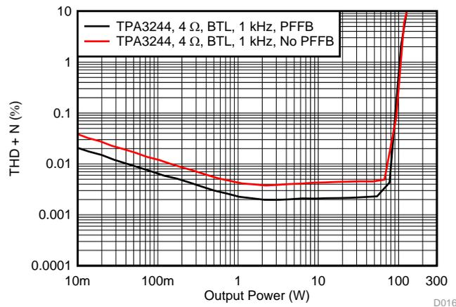
**Figure 25. THD+N vs Power at 1 kHz**
