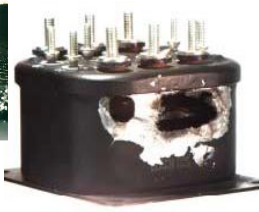
Relay failure due to whisker induced plasma arcing at atmospheric conditions
