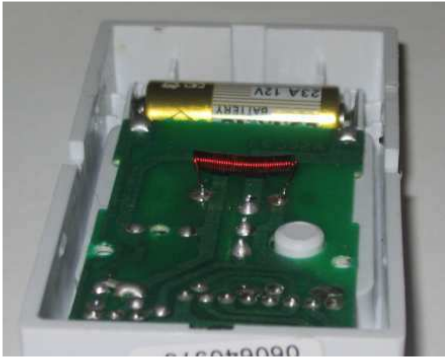
40 turn coil replacing the 1.5uH inductor
