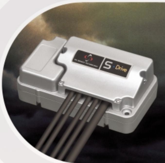
The space available on any scooter is often at a premium. Therefore, to minimise the spatial requirements of the controller, the S120 and S140 battery and motor connectors are recessed on top of the unit, making efficient use of the available area and decreasing the total volume required for the controller and its associated wiring.
