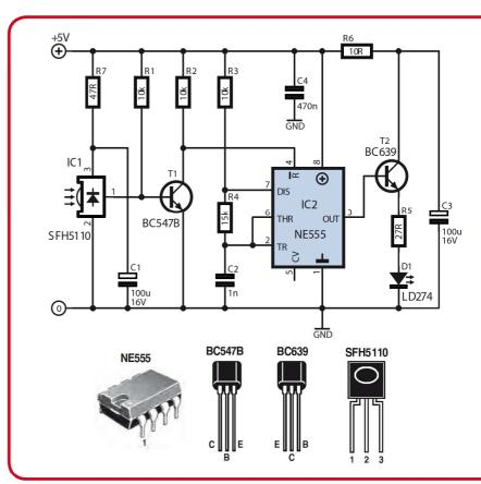
its output goes low and the collector of T1 goes high. This signal drives the Reset input of the timer IC (IC2), which acts as a controlled 36-kHz signal source.
