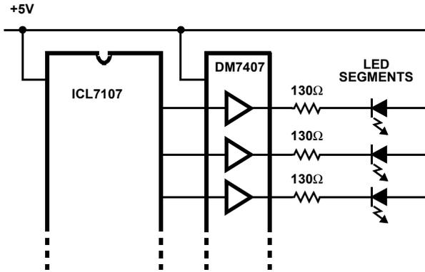
FIGURE 22. DISPLAY BUFFERING FOR INCREASED DRIVE CURRENT
