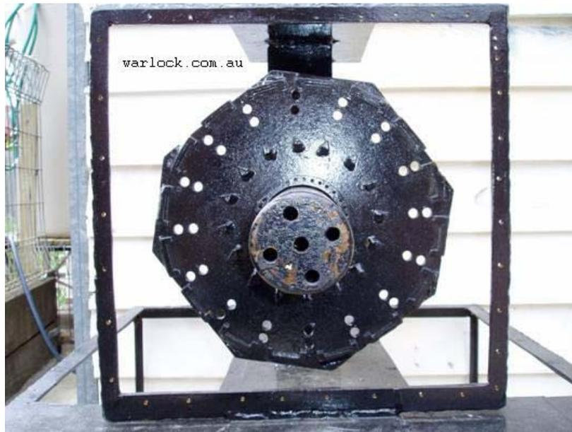
Figure 1. Rear half of the generator rotor
