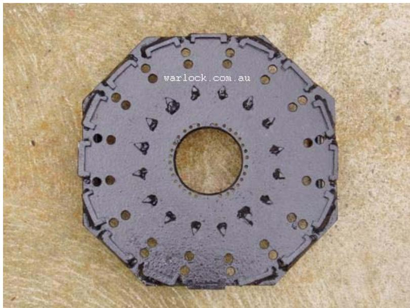
Figure 2. Front half of generator rotor
