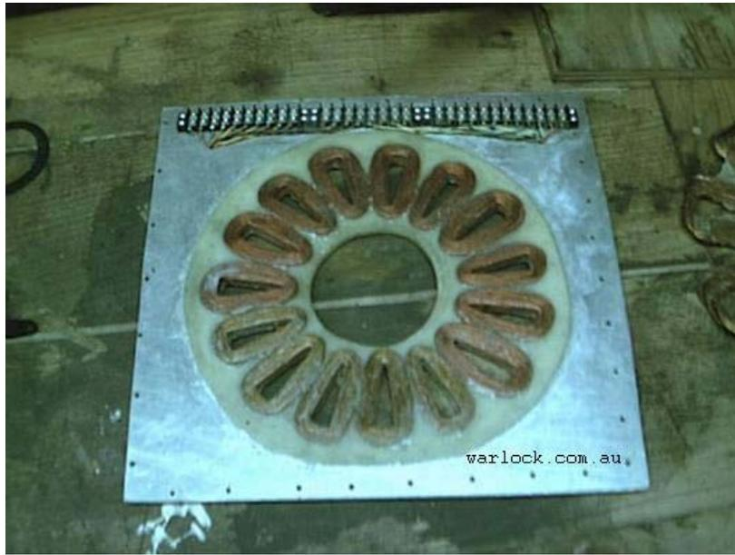
Figure 3. Generator stator
