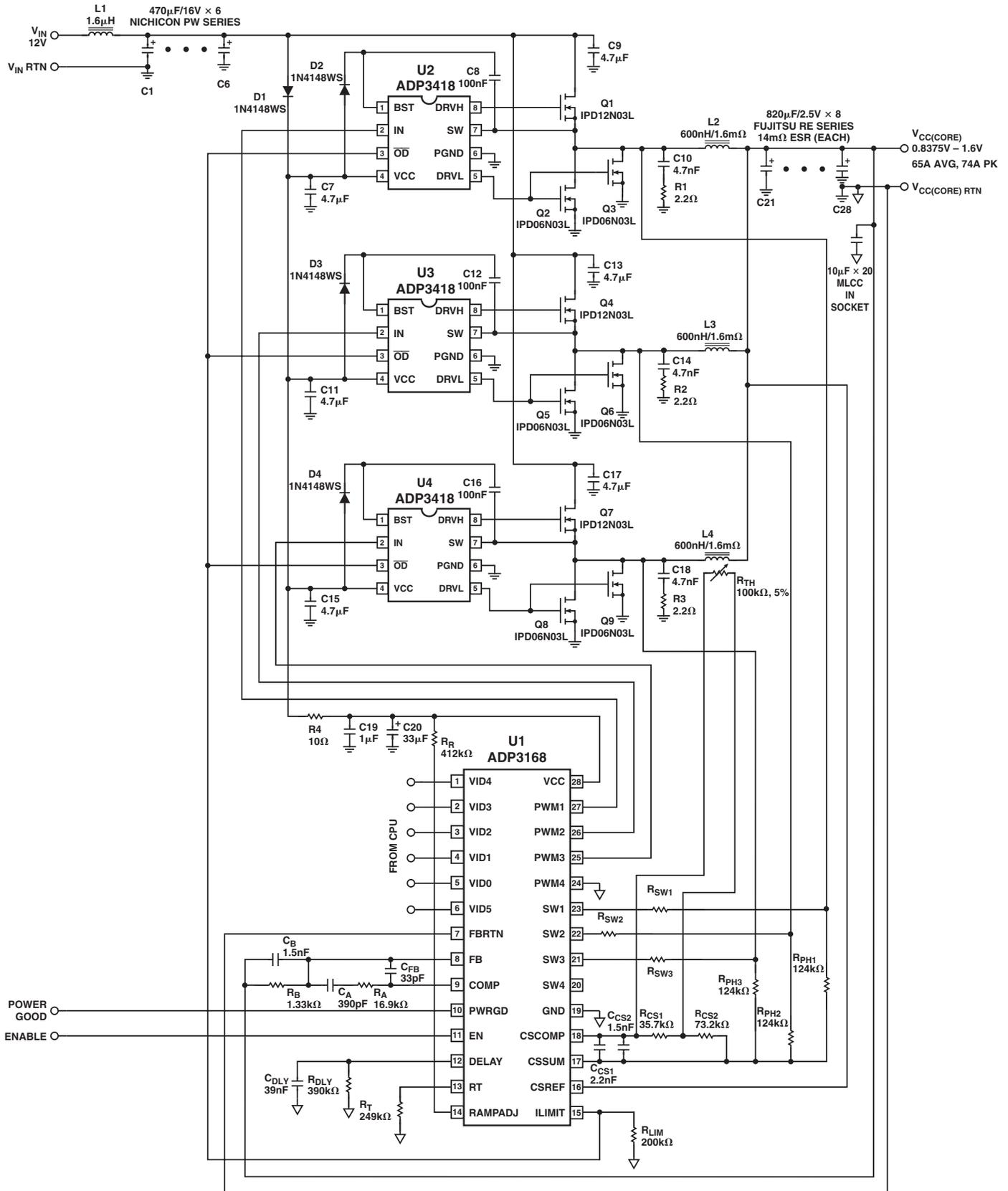
Figure 4. VRD 10 Compliant Intel CPU Supply Circuit
