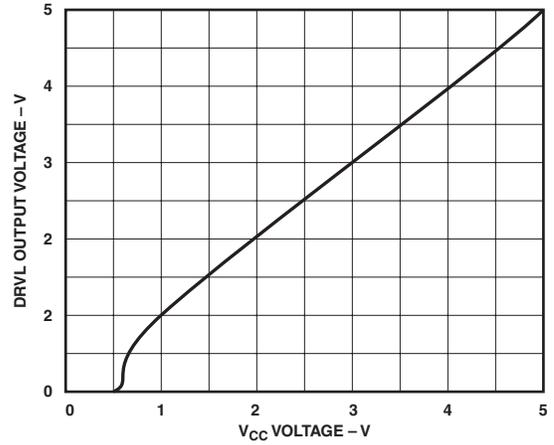
TPC 9. DRV1 Output Voltage vs. Supply Voltage
