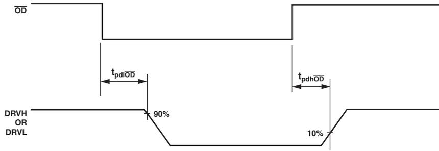
Figure 2. Output Disable Timing Diagram
