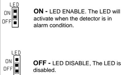
**Note:** The LED Switch does not affect the operation of the relay. When an intrusion is detected, the LED will activate and the alarm relay will switch into alarm condition for 2 sec.
