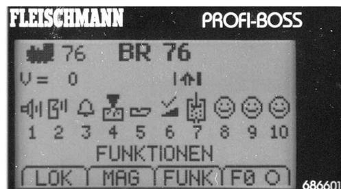
The tick over the pictogram symbol "ramp" will now change to a "cross" = off. (pressing the key "6" again will switch the inertia back on again).
