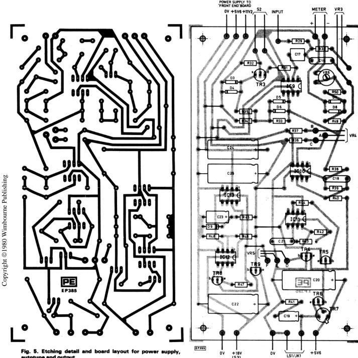
Fig. 5. Etching detail and board layout for power supply, autotune and output
