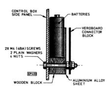
Fig. 9 (left). Control fascia; (above) Detail of battery mounting
