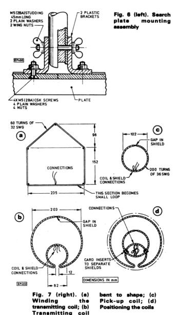
were cut from a thick, strong square-shaped clip intended for mounting square section plastic drain pipes to exterior walls, obtained from a local builders' merchants. They are bolted to the plate with 2BA countersunk screws with the heads inside, so nothing protrudes to foul the coils. A hole is drilled just behind one of the brackets to allow a 4core screened cable to pass through.
