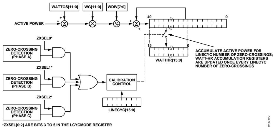
Figure 70. ADE7758 Line Cycle Active Energy Accumulation Mode
