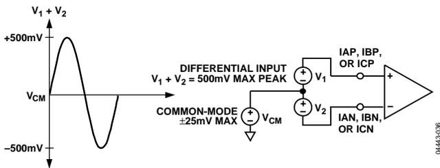
Figure 36. Maximum Signal Levels, Current Channels, Gain = 1
