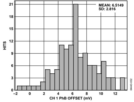
Figure 32. Phase B Channel 1 Offset Distribution
