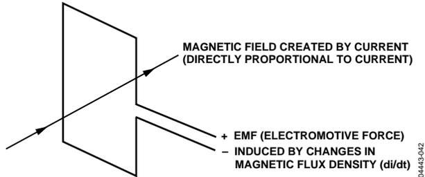
Figure 42. Principle of a di/dt Current Sensor
