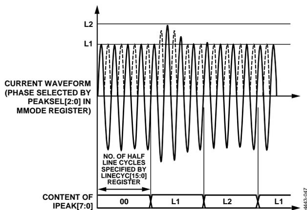
Figure 47. Peak Current Detection Using the IPEAK Register
