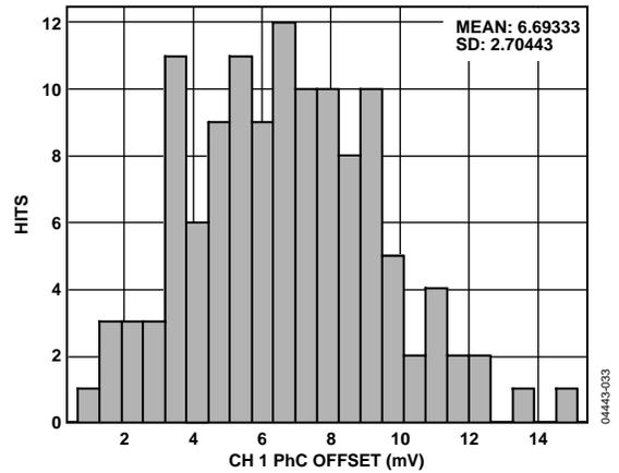
Figure 33. Phase C Channel 1 Offset Distribution
