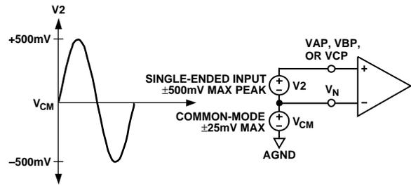
Figure 37. Maximum Signal Levels, Voltage Channels, Gain = 1
