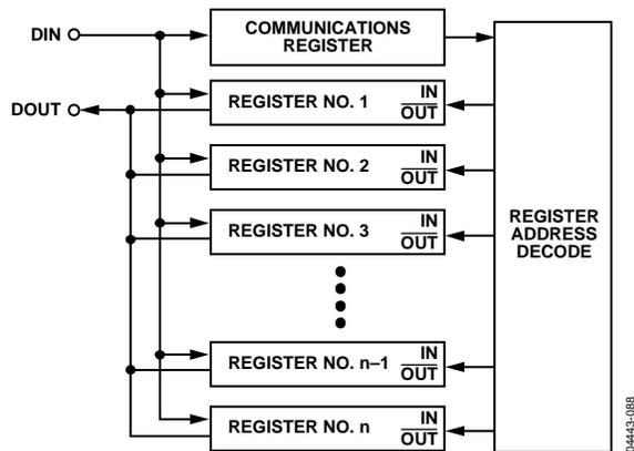
Figure 88. Addressing ADE7758 Registers via the Communications Register
