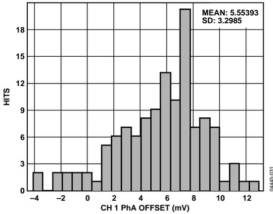
Figure 31. Phase A Channel 1 Offset Distribution
