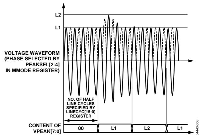
Figure 58. Peak Voltage Detection Using the VPEAK Register
