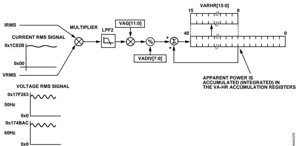
Figure 75. ADE7758 Apparent Energy Accumulation
