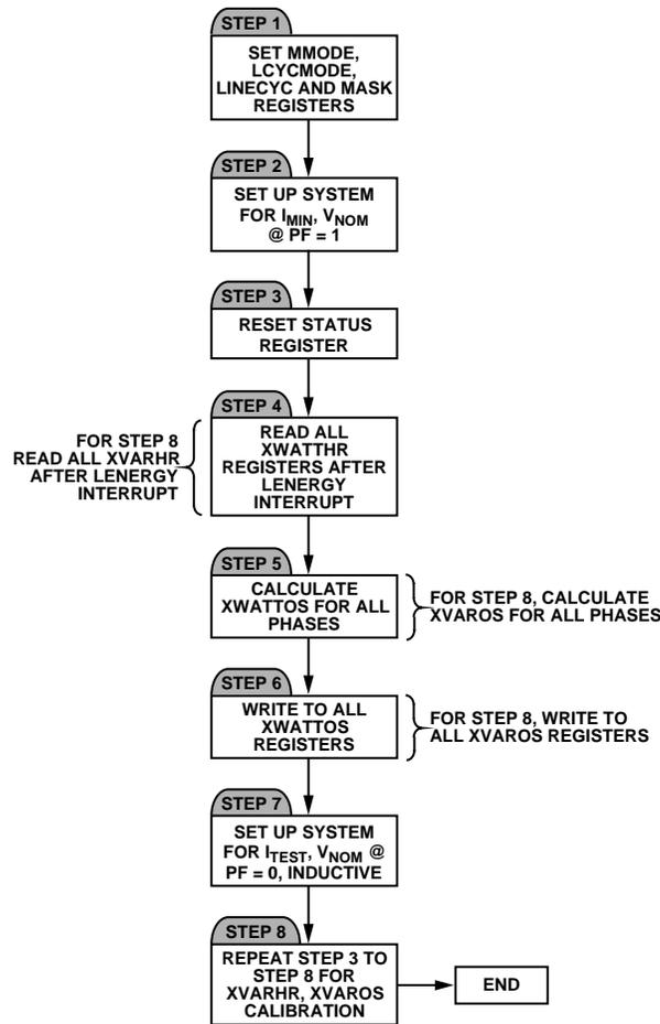
Figure 83. Power Offset Calibration Using Line Accumulation
