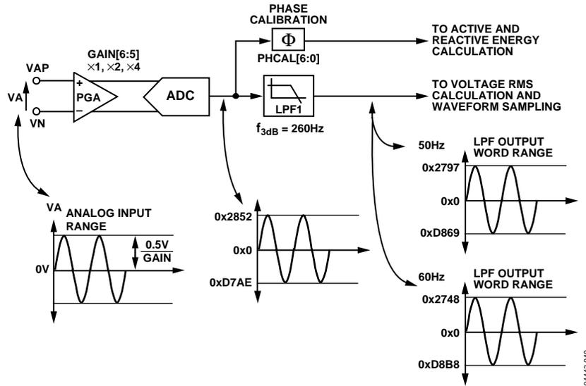
Figure 49. ADC and Signal Processing in Voltage Channel
