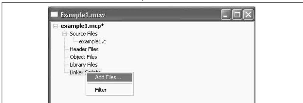
Use the linker script 18f452.lkr in the lkr subdirectory of the MPLAB C18 installation directory. This script is for the PIC18F452 device.
