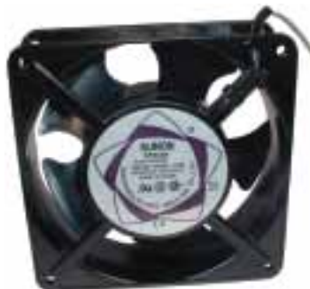
DP203A-2123LSL i GES 071 000 28 Ventilátor SUNON 230VAC/11VA, 2000ot, 118m 3 /h, 36dB, 120x120x38mm, 550g
