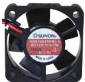
KDE1204PFB1-8 i GES 071 000 31 Vent. kuličkový SUNON 12VDC/0,6W, 6100ot, 10m 3 /h, 28dB, 40x40x10mm
