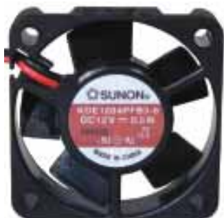
KDE1204PFB1-8 i GES 071 000 31 Vent. kuličkový SUNON 12VDC/0,6W, 6100ot, 10m 3 /h, 28dB, 40x40x10mm
