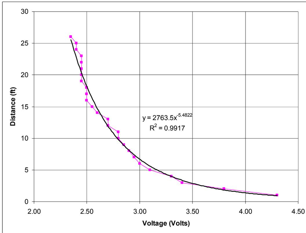
Figure 5 - Plot used for the voltage to distance calculation
