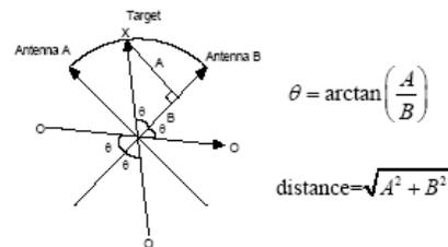
Figure 1 - Direction analysis diagram. X represents the true target location and O represents false target locations.
