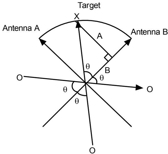
Figure 6 - Direction analysis diagram. X represents the true target location and O represents false target locations.
