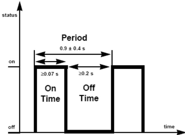
Figure 3 - ETS 300 718 standard on pulse periods and pulse widths
