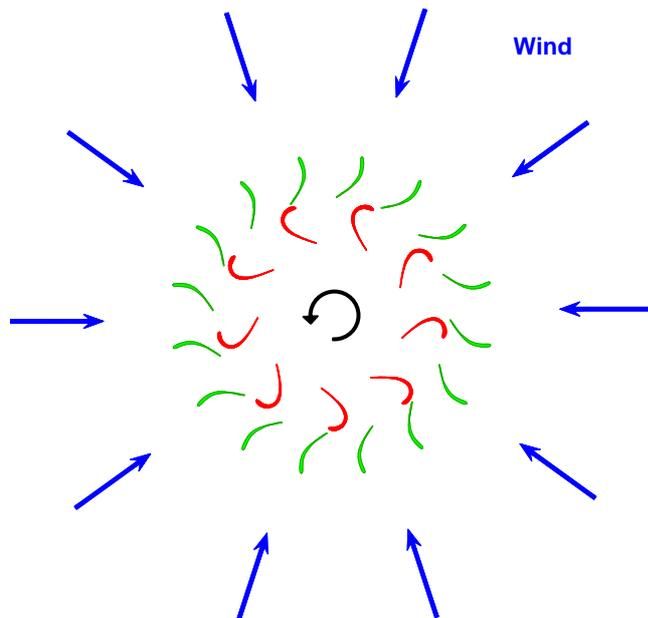
The axisymmetry of the STATOEOLIEN enables it to be totally independent from the wind direction changes. Indeed, the fixed wings of the stator and the moving blades of the rotor are distributed in a symmetrical way around the vertical shaft of the machine, thus supporting no privileged operating direction. The result is an optimal working whatever the wind direction, which is particularly useful with urban winds, that are characterized by frequent direction changes.
