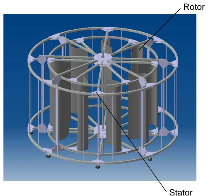
3/ When the rotor blades expose their leeward side to the wind, they generate a torque that will oppose the normal working rotation. This results in power loss. Therefore the stator has been designed to generate in this "brake" zone turbulences that will prevent wind from entering the machine and pushing the blades in the wrong direction, thus reducing this braking effect.
