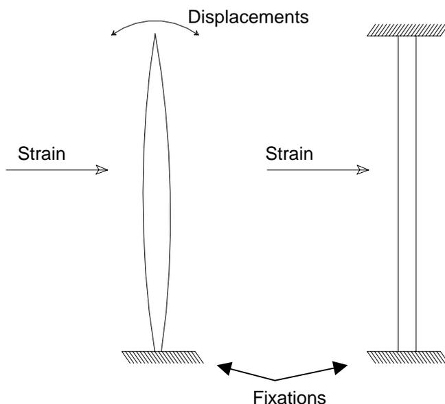
Comparison between a cantilever structure (left hand) and a structure fixed at both ends (right hand). The first one is mechanically unstable (vibrations, high stress constraints applied to fixations). On the other hand, the second one transmits the efforts and vibrations to both fixations, leading to maximum stability.
