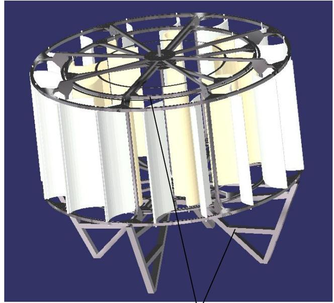
Painted steel (stator) and aluminium (rotor) tubular structures
