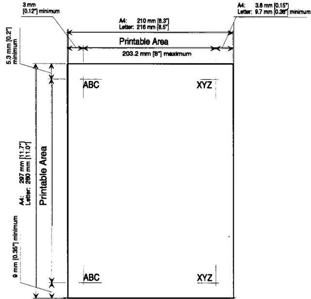
**Figure 1-3. Printable Area for Cut Sheets Using the CSF**
