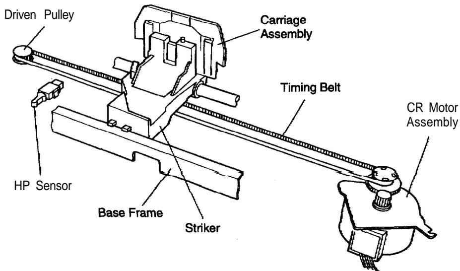
**Figure 2-2. Carriage Movement Mechanism**
