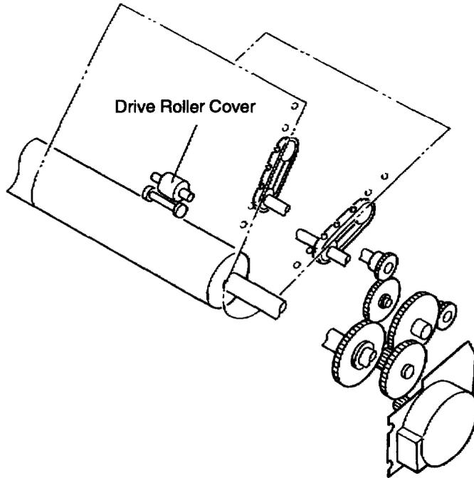
**Figure 2-6. Push-Pull Tractor Paper Advance Mechanism**
