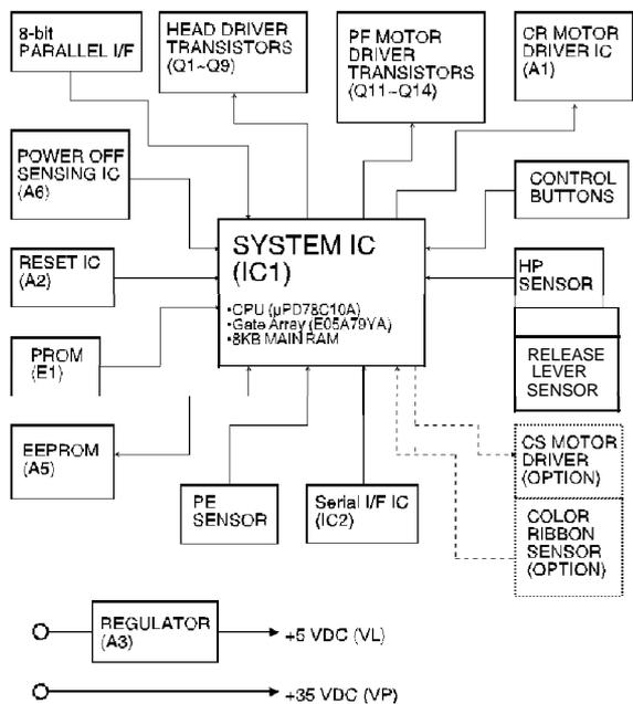
**Figure 2-12. Control Circuit Block Diagram**
