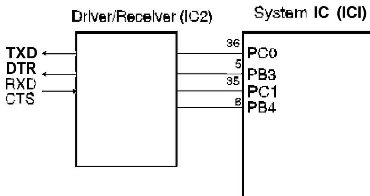
Figure 2-21. Serial Interface Block Diagram
