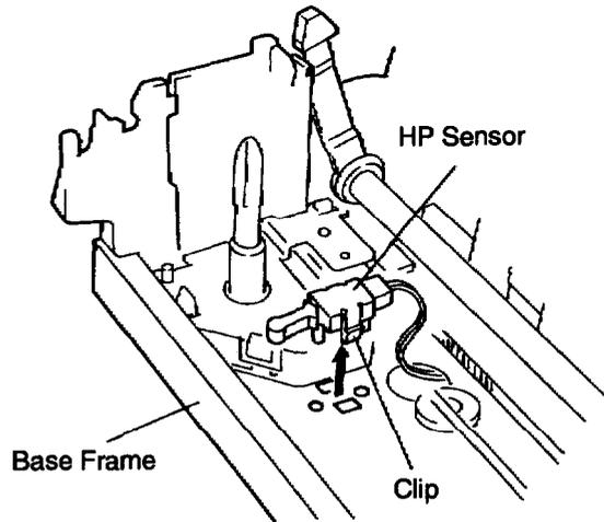
Figure 3-14. Removing the HP Sensor
