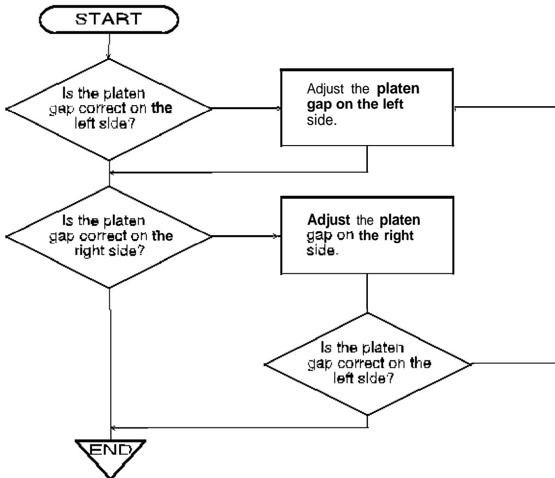
Figure 4-1. The Flowchart for the Platen Gap Adjustment
