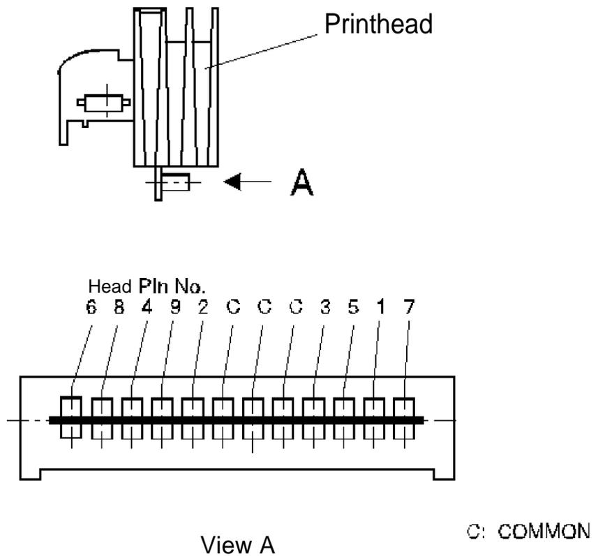
**Figure 5-1. Printhead Connector Pin Alignment**
