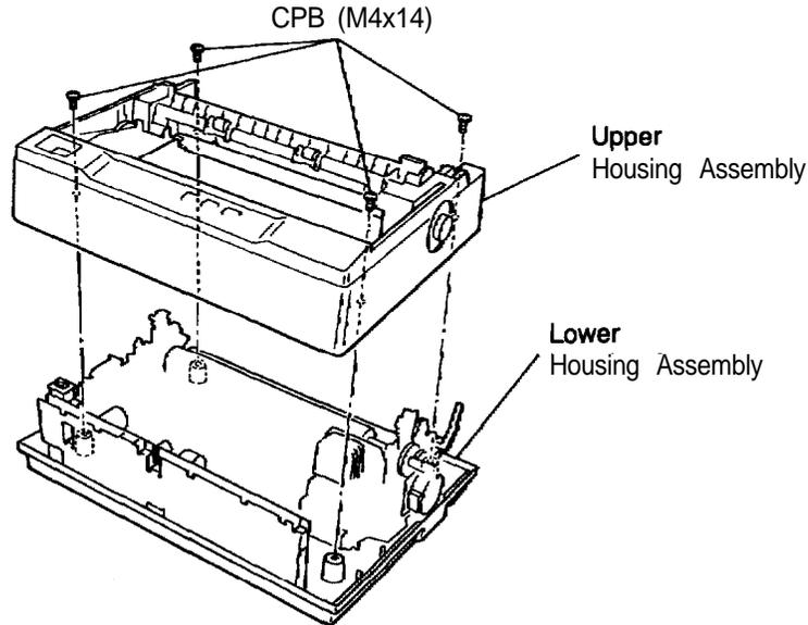
Figure 3-3. Removing the Upper Housing Assembly
