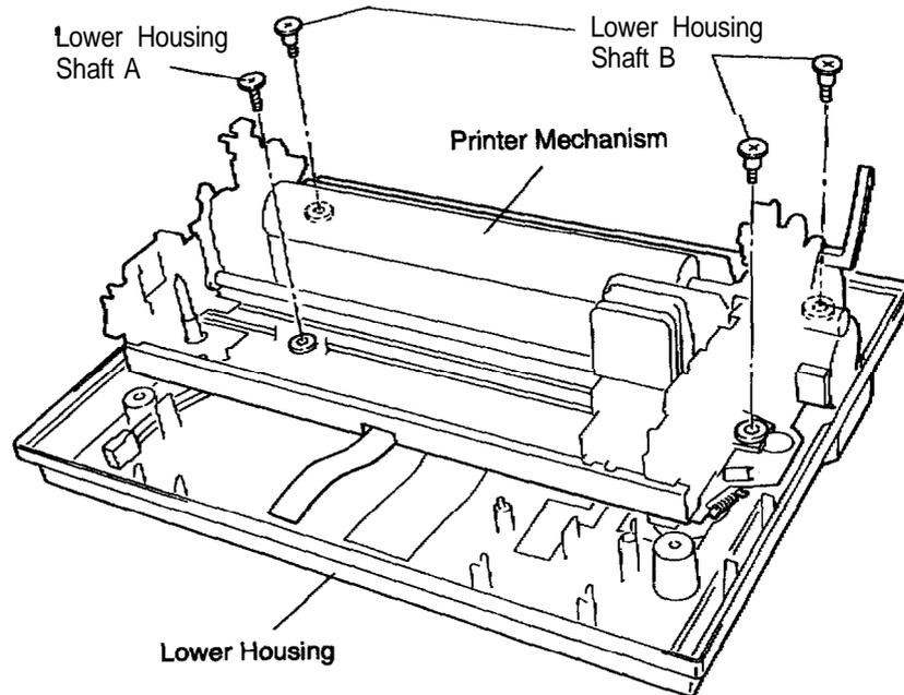
**Figure 3-8. Removing the Printer Mechanism**
