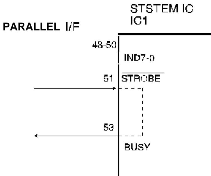
Figure 2-20. Parallel Interface Block Diagram
