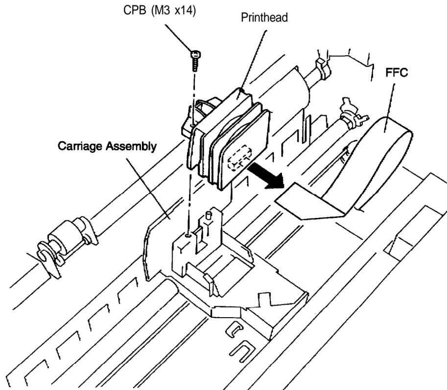
Figure 3-2. Removing the Printhead
