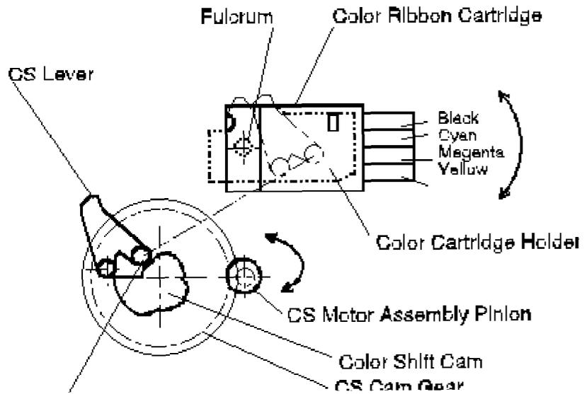
Figure 2-9. Color Shift Mechanism
