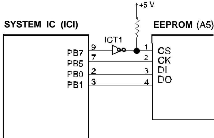
Figure 2-22. EEPROM Control Circuit Diagram
