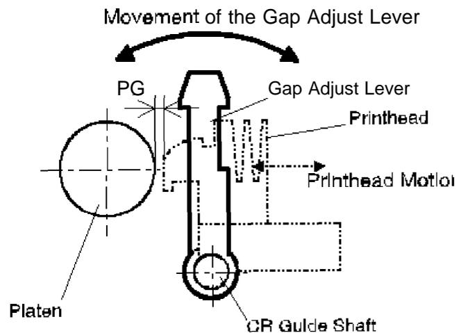
Figure 2-10. Platen Gap Adjustment Mechanism
