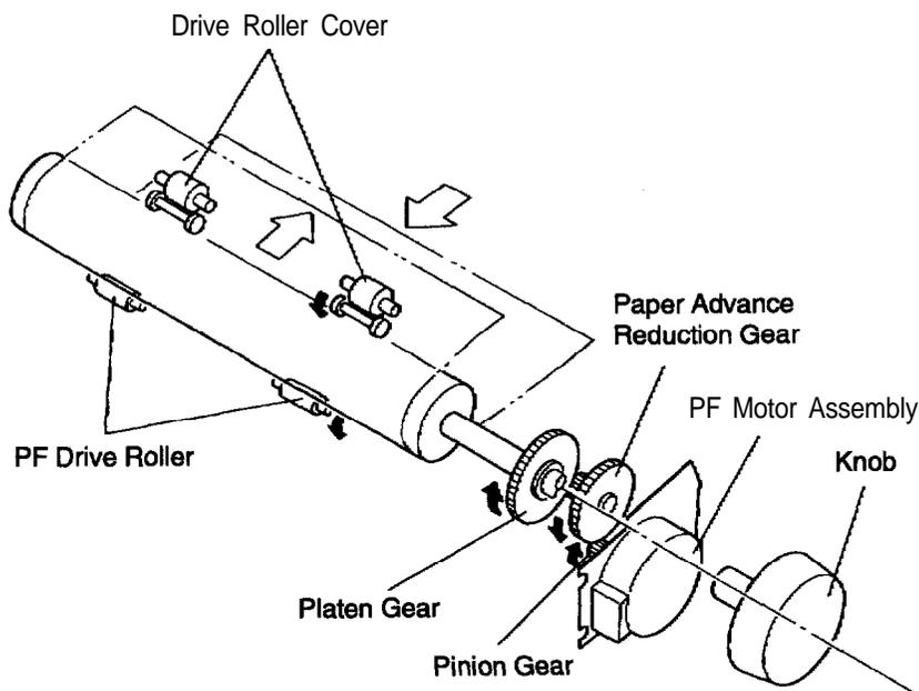
Figure 2-3. Friction Advance Mechanism
