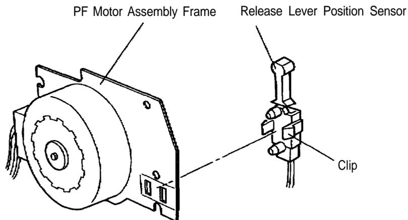
Figure 3-15. Removing the Release Lever Position Sensor
