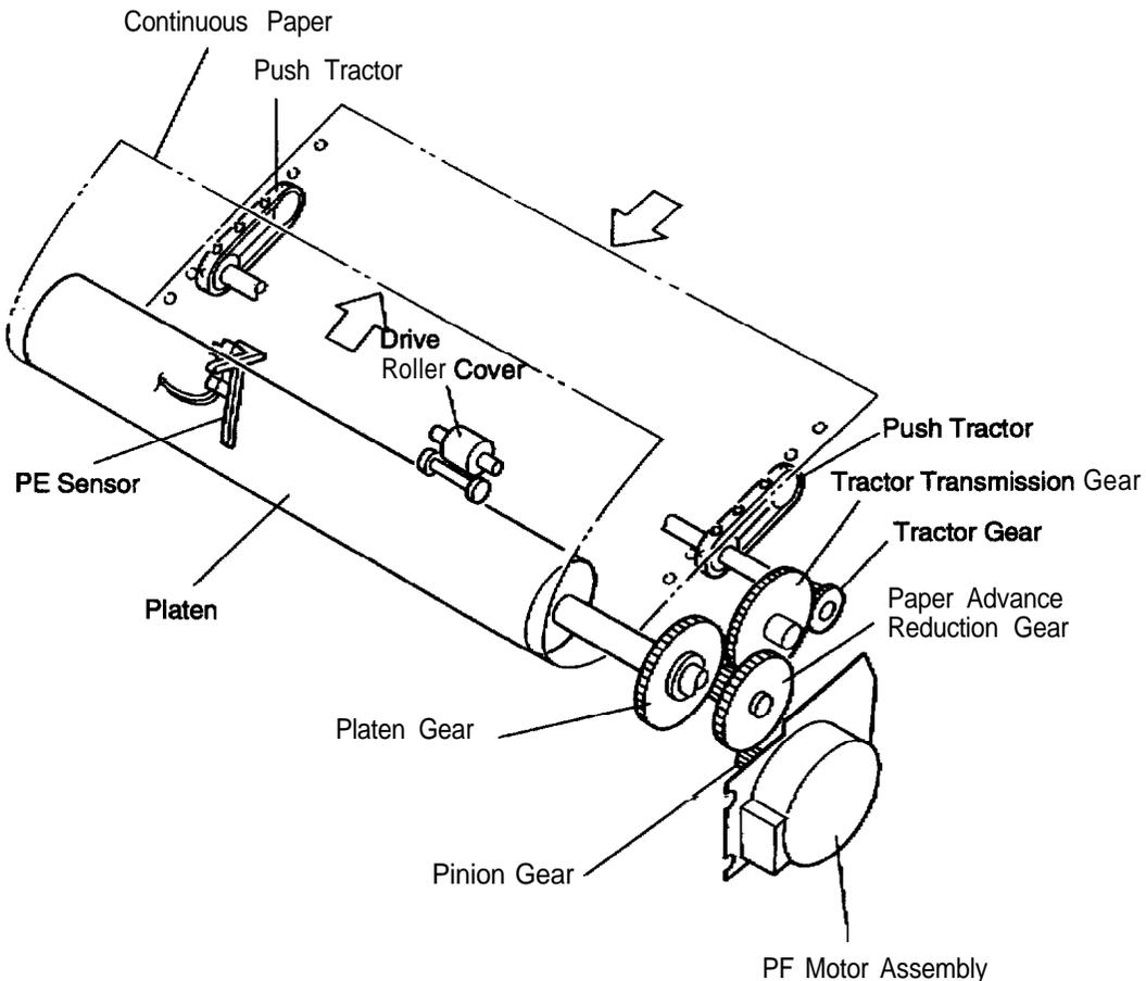
Figure 2-4. Push Tractor Paper Advance Mechanism
