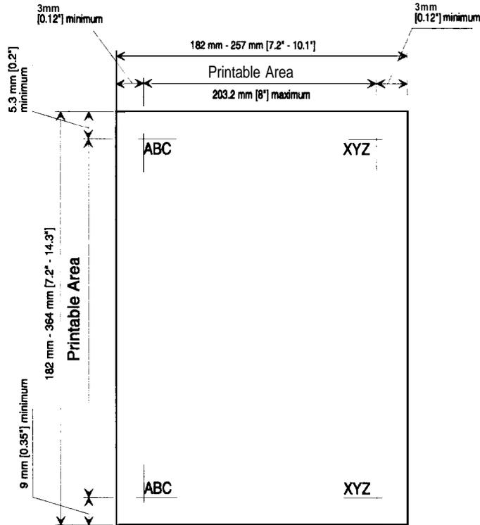
**Figure 1-4. Printable Area for Cut Sheets Using Manual Insertion**
