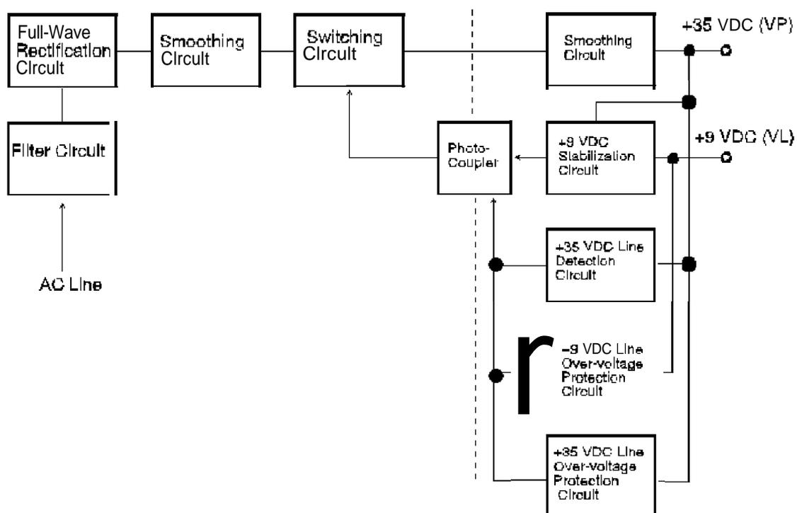
Figure 2-11. Power Supply Circuit Block Diagram
