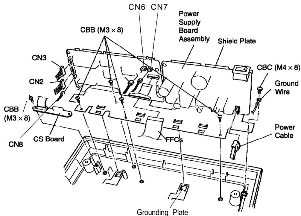
Figure 3-5. Removing the Shield Plate
