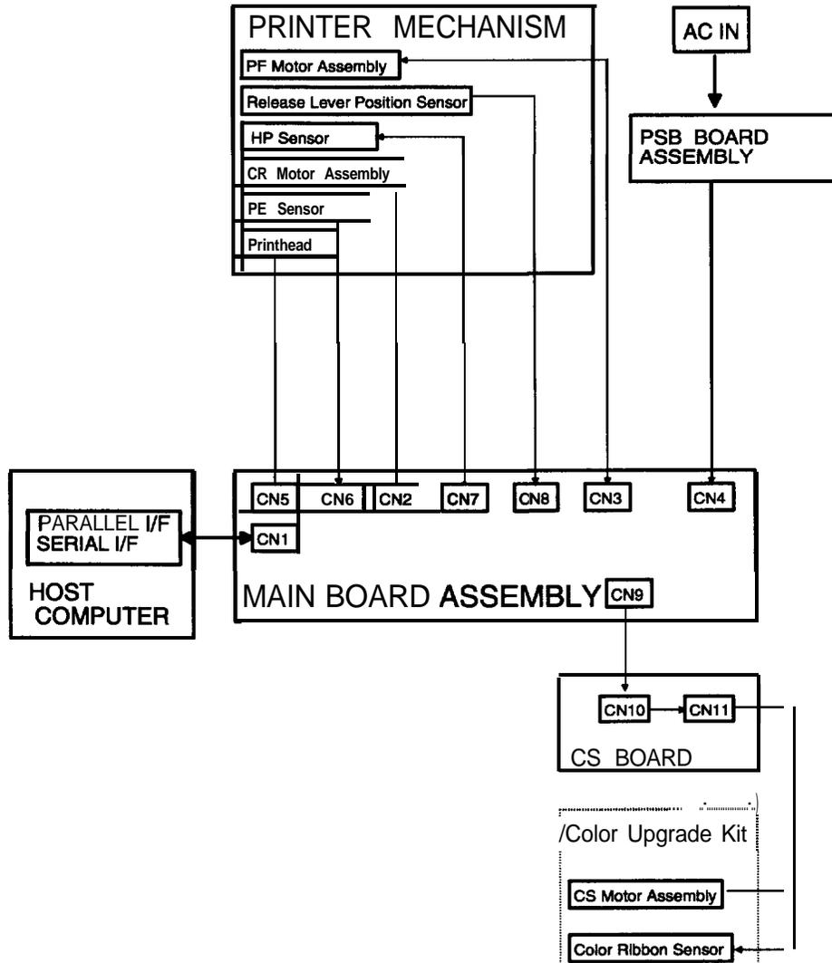
Figure A-1. Cable Connections
