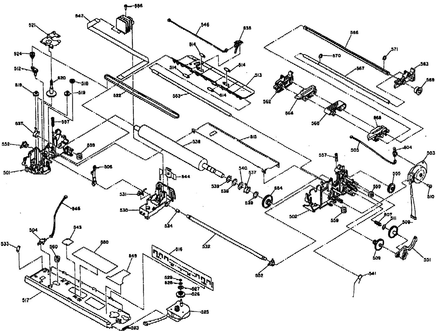
Figure A-6. LX-300 Exploded Diagram
