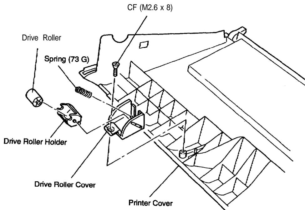
**Figure 3-19. Removing the Drive Roller Assembly**
