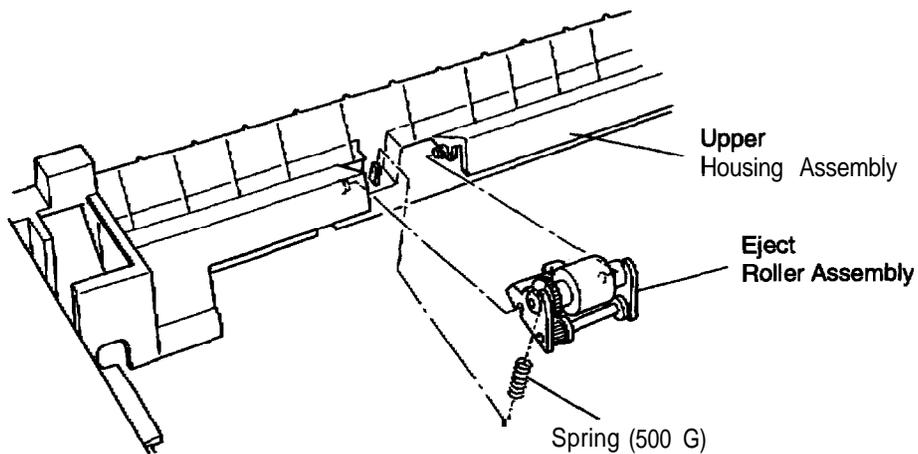
Figure 3-4. Removing the Eject Roller Assembly
