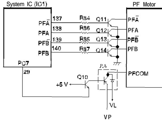
Figure 2-18. Paper Feed Motor Driver Circuit Diagram
