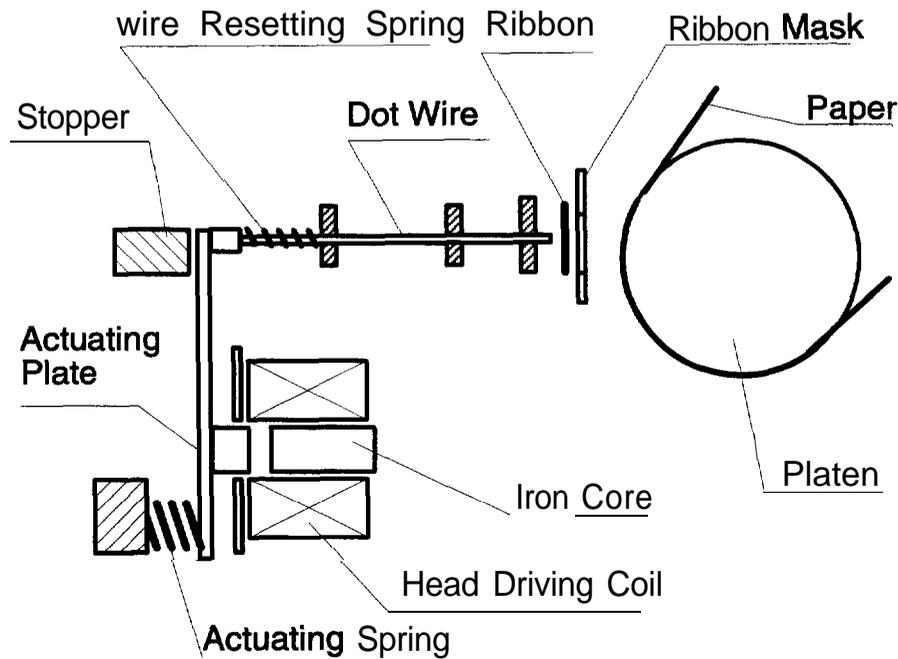
Figure 2-1. Printhead Operation Principles
