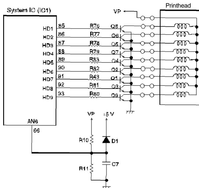
Figure 2-19. Printhead Driver Circuit Diagram
