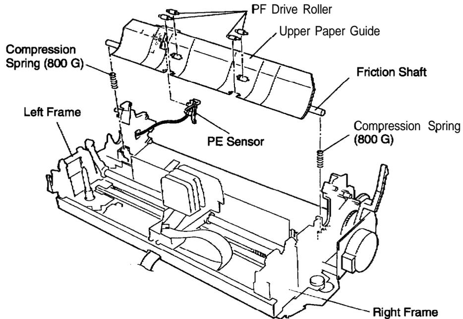
Figure 3-12. Removing the PE Sensor
