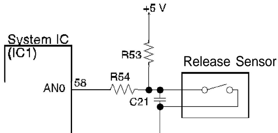
Figure 2-16. Release Lever Position Sensor Circuit Diagram
