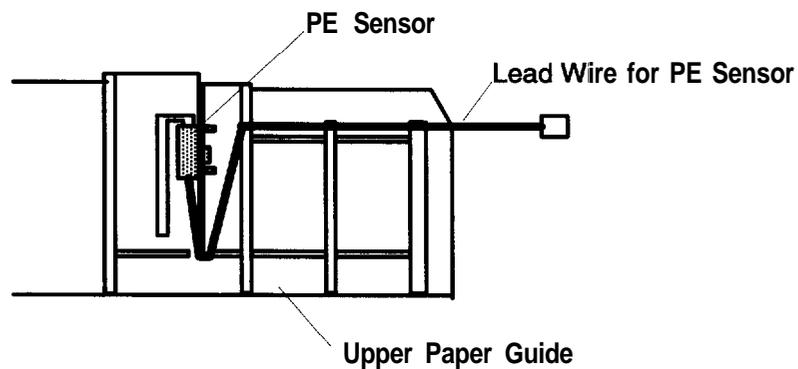
Figure 3-13. Wiring of the PE Sensor
