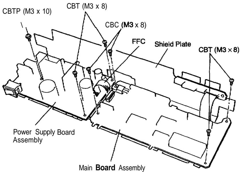
Figure 3-6. Removing the Main Board Assembly and PSB
