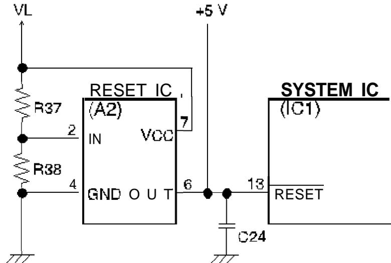
Figure 2-13. Power On Rest Circuit Diagram
