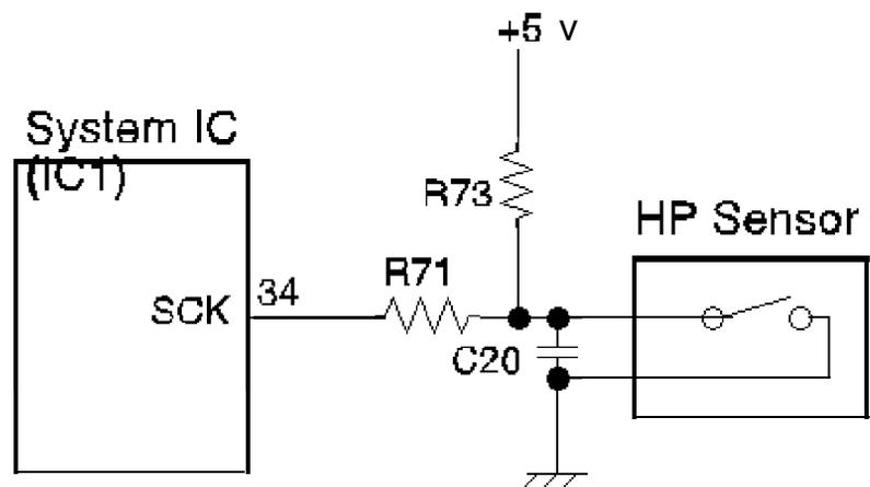
Figure 2-14. Home Position Sensor Circuit Diagram
