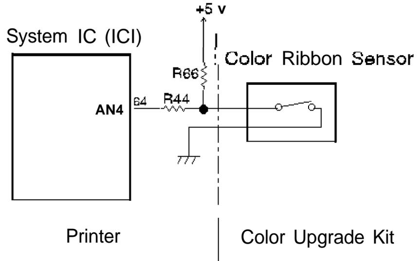
Figure 2-24. Color Ribbon Sensor Circuit Diagram
