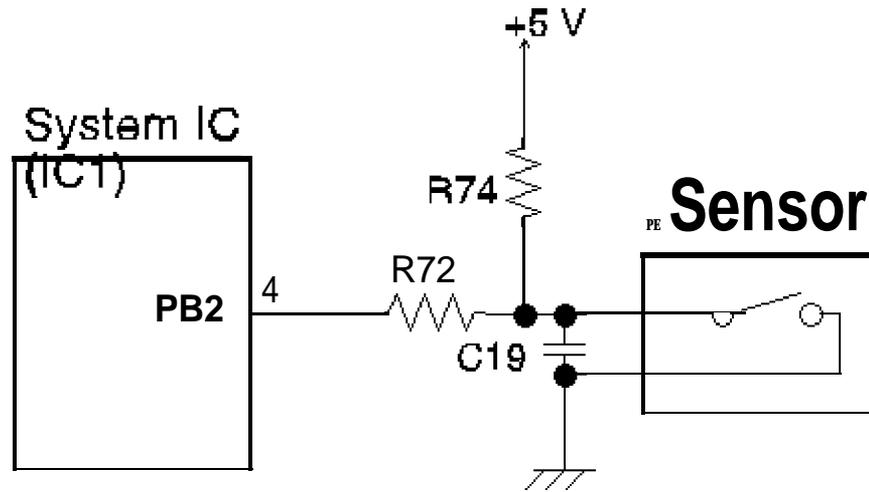
Figure 2-15. Paper End Sensor Circuit Diagram
