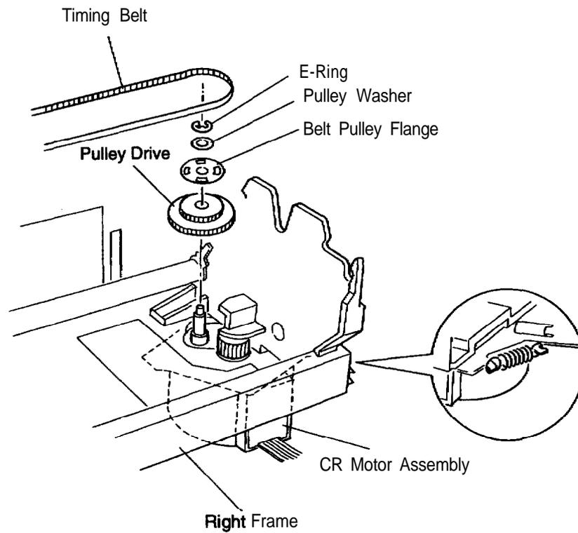
Figure 3-10. Removing the CR Motor Assembly
