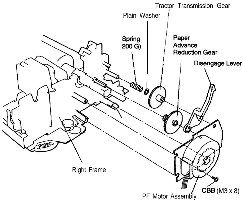
**Figure 3-9. Removing the PF Motor Assembly**
