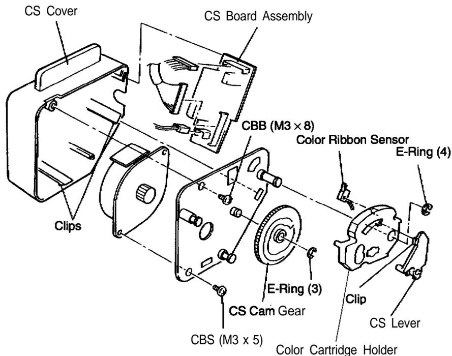
Figure 3-20. Disassembling the Optional Color Upgrade Kit
