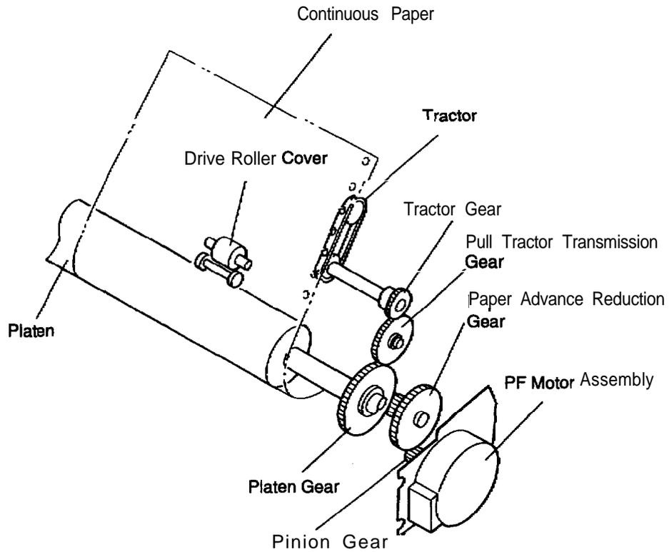
**Figure 2-5. Pull Tractor Paper Advance Mechanism**
