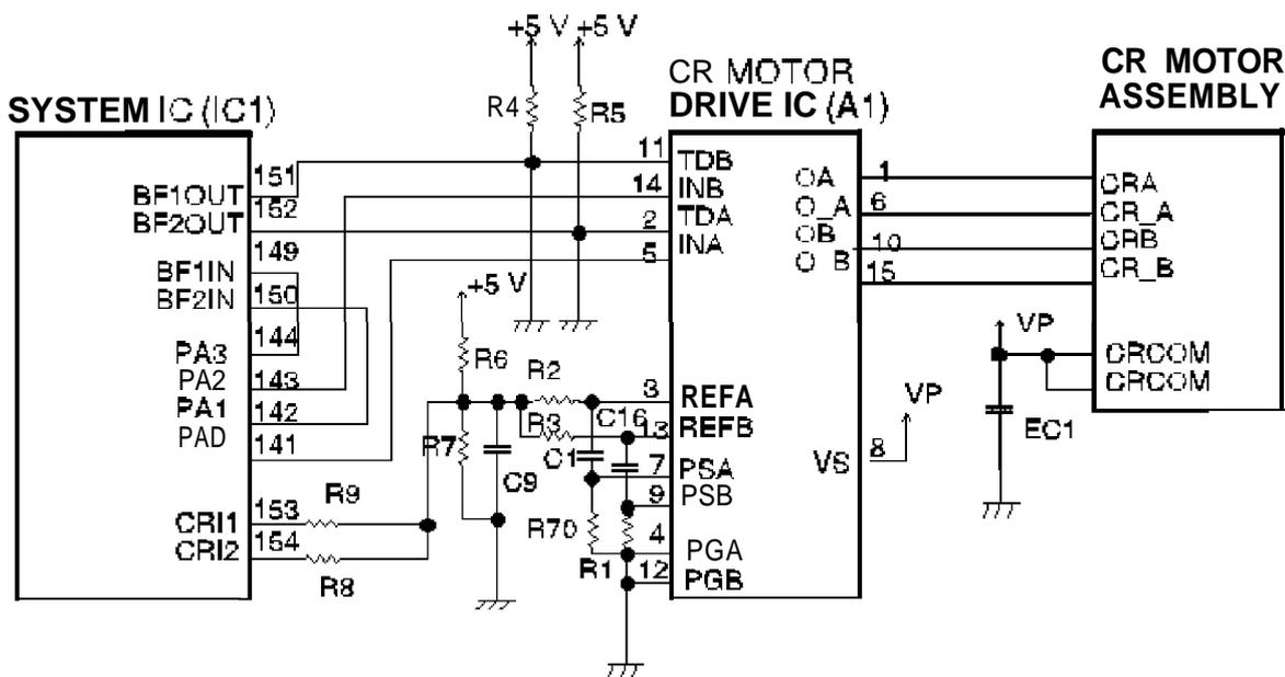
**Figure 2-17. Carriage Motor Driver Circuit**
