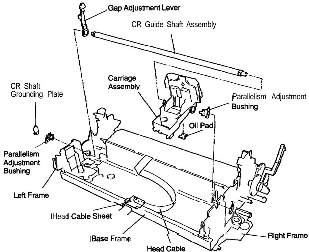
Figure 3-18. Removing the Carriage Assembly
