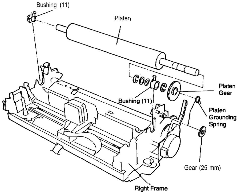
Figure 3-11. Removing the Platen
