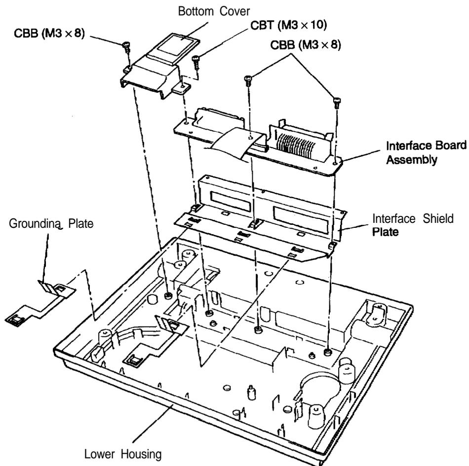
Figure 3-18. Removing the Interface Board Assembly
