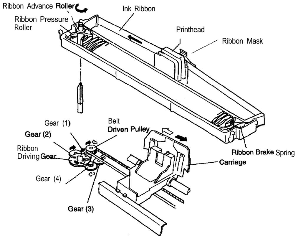
**Figure 2-6. Ribbon Advance Gear Linkage**
