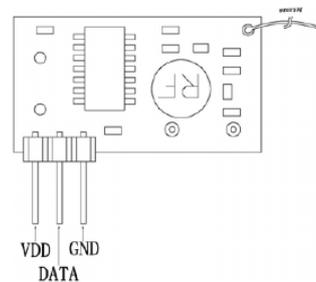
IF DATA pin is idle for more than 70mS, then the module will enter standby mode automatically.
