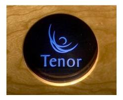
The lens on the front panel is an indicator light that is dark (i.e. not lit), red or blue and, in the event of a fault, blue will change to red in 1-second increments.
