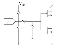
Note 4 : Output equivalent circuit
