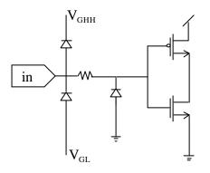
Note 5 : Input equivalent circuit
