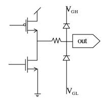
Note 6 : Output equivalent circuit
