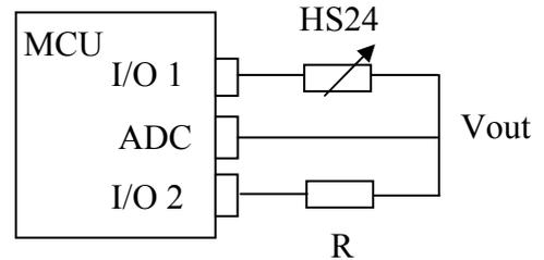
To prevent polarization of the sensor, resistive sensors use symmetrical AC excitation voltage with no DC bias. In this method, AC excitation is generated and managed by microcontroller I/O.
