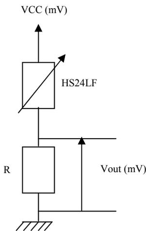
$$V_{out} (mV) = \frac{VCC (mV) * R (\Omega)}{R (\Omega) + HS24LF (\Omega)}$$
