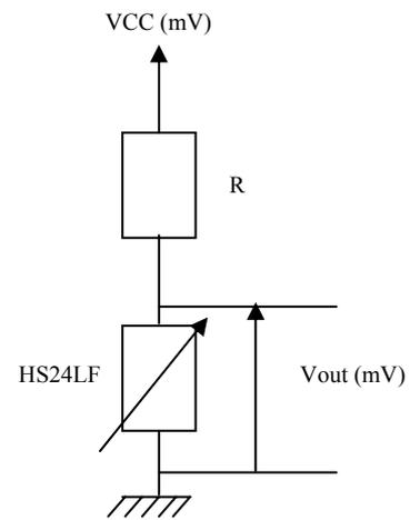
$$V_{out} (mV) = \frac{VCC (mV) * HS24LF (\Omega)}{R (\Omega) + HS24LF (\Omega)}$$
