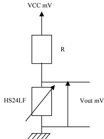
$$V_{out} (mV) = \frac{VCC (mV) * HS24LF (\Omega)}{R (\Omega) + HS24LF (\Omega)}$$
