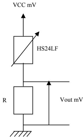
$$V_{out} (mV) = \frac{VCC (mV) * R (\Omega)}{R (\Omega) + HS24LF (\Omega)}$$
